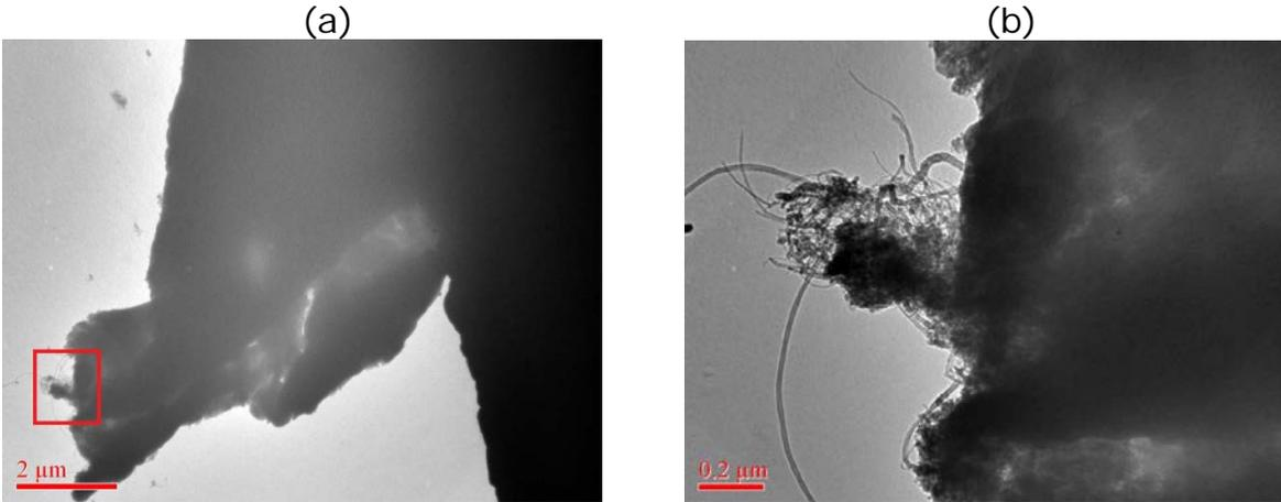
Figure 10. TEM images from the filter sample collected in the ball milling room: (a) CNT matrix, and (b) closer view of Figure 10-a.
