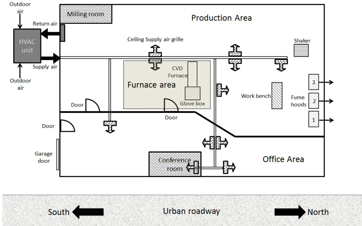
Figure 1. Plant layout showing ventilation distribution details and location of operations and fume hoods.
