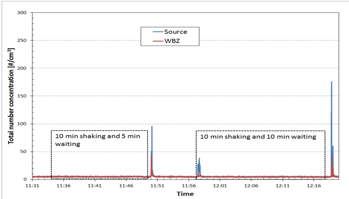
Figure 8. Monitoring data for the sieve shaking process on Day 2: (a) DustTrak data and (b) OPS data.
