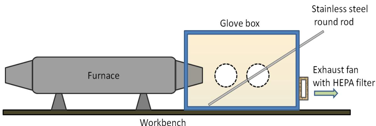
Figure 2. CNT production system. A ventilated glove box was installed at the unloading port of the furnace for product harvest.
