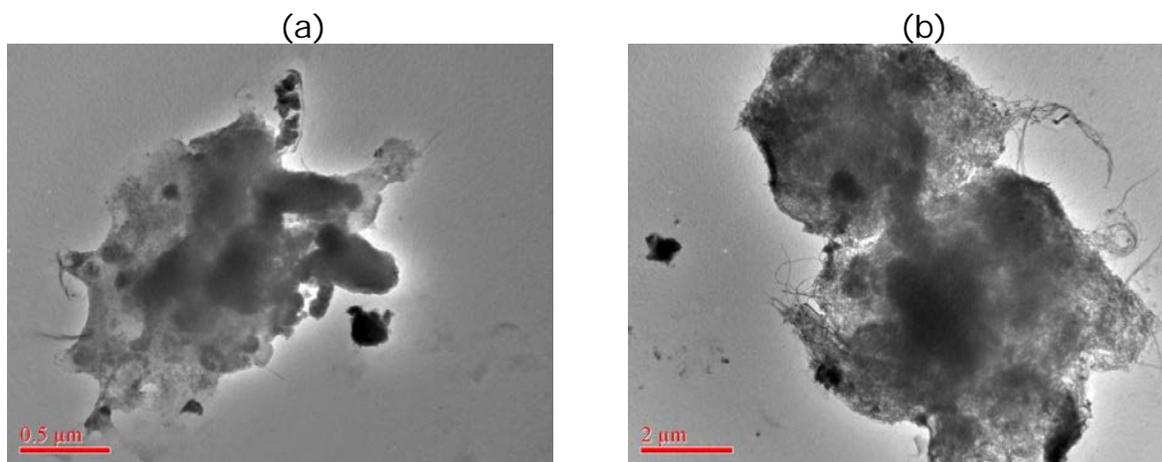
Figure 9. TEM images from the filter sample collected at top of the cabinet for the sieve shaking process: (a) CNT matrix, and (b) CNT cluster.
