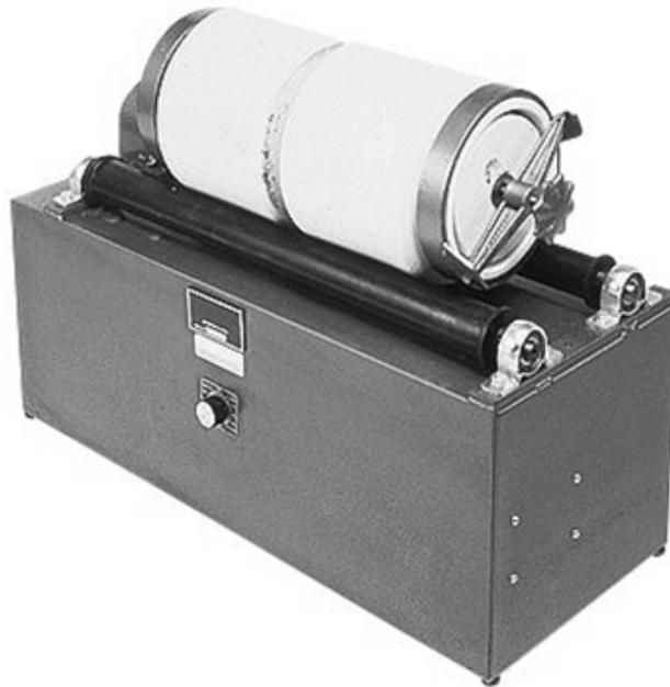
Figure 4. A high-capacity laboratory jar on a roller. The study site used similar equipment to grind nanomaterials (photo source: <http://www.coleparmer.com/buy/product/52775-one-tier-jar-high-capacity-laboratory-jar-mill-24-roller-115-vac-60-hz.html>).
