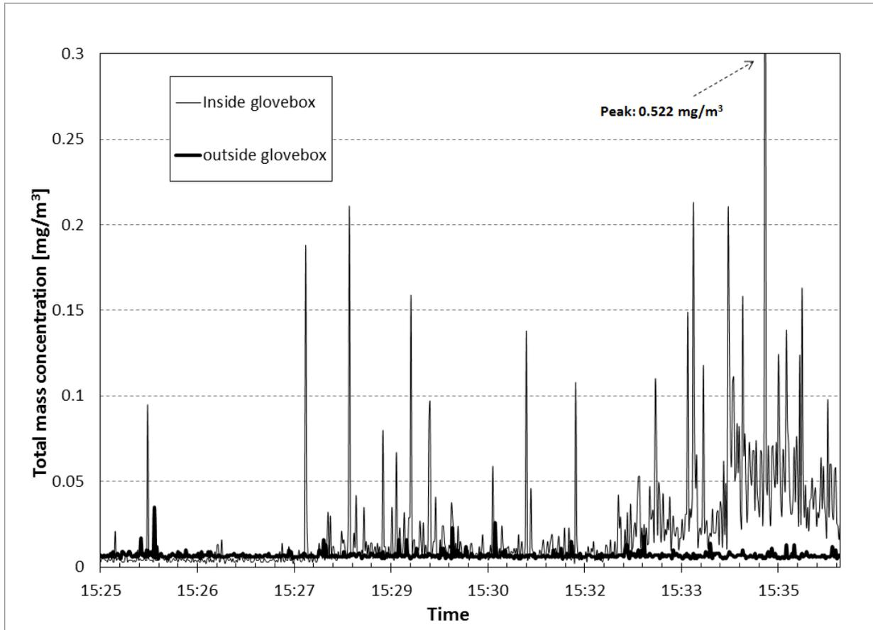
Figure 5. Monitoring data from two SidePaks located inside and outside the glove box during product harvest.
