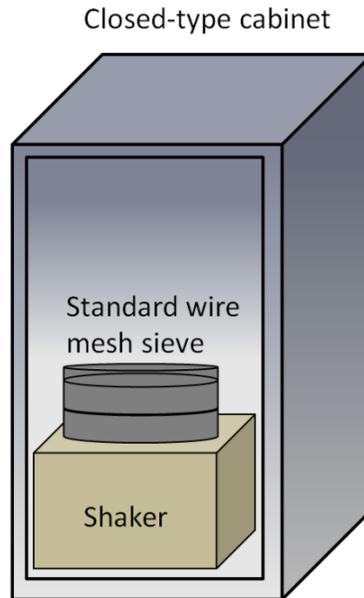
Figure 3. Sieving process. The process was done by shaking standard wire mesh sieves inside a closed cabinet without any local ventilation.
