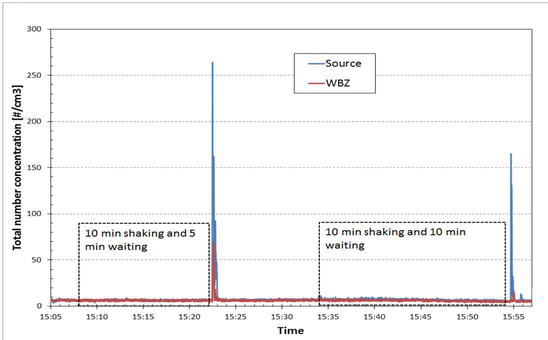
Figure 7. Monitoring data for the sieve shaking process on Day 1: (a) DustTrak data and (b) OPS data.
