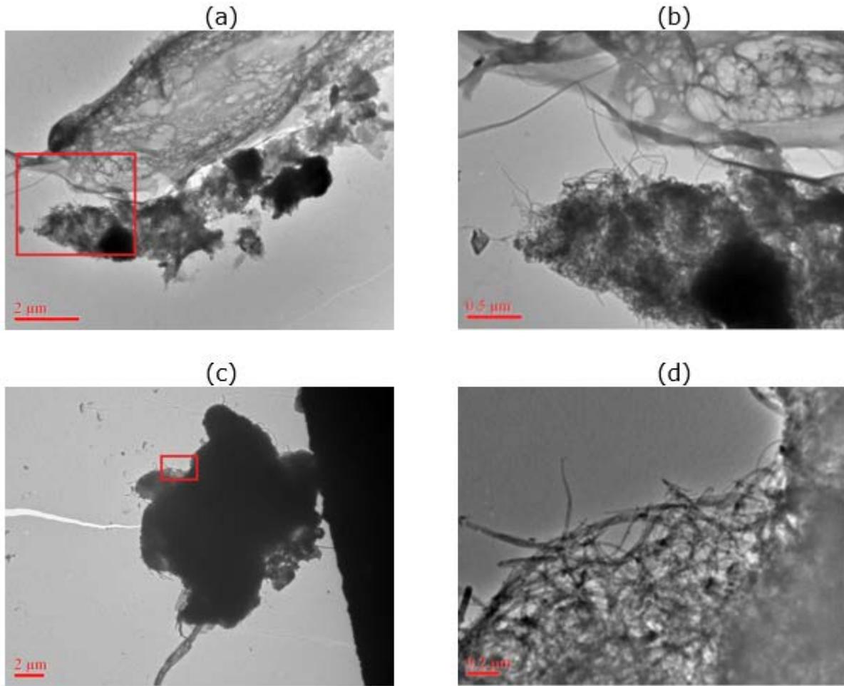
Figure 6. TEM images from the filter sample collected near the production furnace: (a) CNT matrix, (b) closer view of Figure 6-a, (c) another CNT matrix, and (d) closer view of Figure 6-c.
