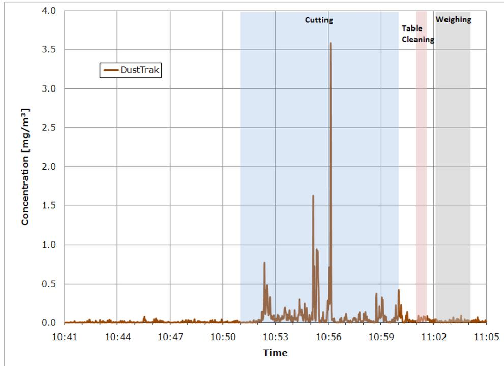
**Figure 15.** Mass concentration variations of the R&D activities monitored by DustTrak on 04/28.
