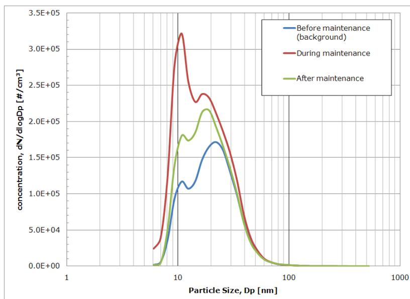
**Figure 8:** Average size distributions during the maintenance task performed at the DARPA Furnace monitored by FMPS 1 on 09/23/2010. The size distribution after maintenance was calculated by the data between 13:45 (starting background check) and 13:49 (reaching the normal background level) as shown in **Figure 7**.
