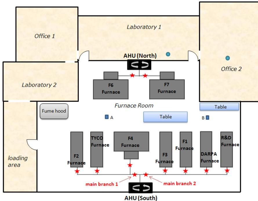
**Figure 1:** Layout of the facility for site survey. Square dots in the furnace room and circular dots in other rooms show the locations for area monitoring. Star symbols indicate the locations where duct velocities and/or air temperatures were measured.
