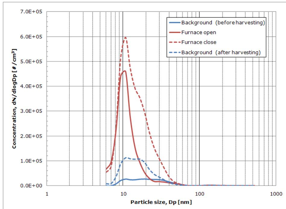
**Figure 11:** Process monitoring by FMPS 1 on 9/23/2010 for product harvesting from Furnace F4; (a) particle concentration over entire process, and (b) average particle size distributions during different stages of F4 product harvesting.
