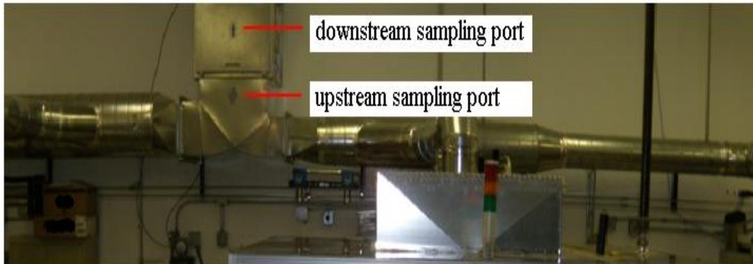
**Figure 5:** Exhaust ventilation system (EVS) where the locations of upstream/downstream sampling ports are shown.
