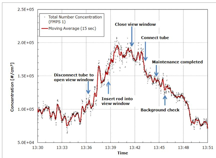
**Figure 7:** Process monitoring by FMPS 1 for the DARPA Furnace during maintenance on 09/23/2010.
