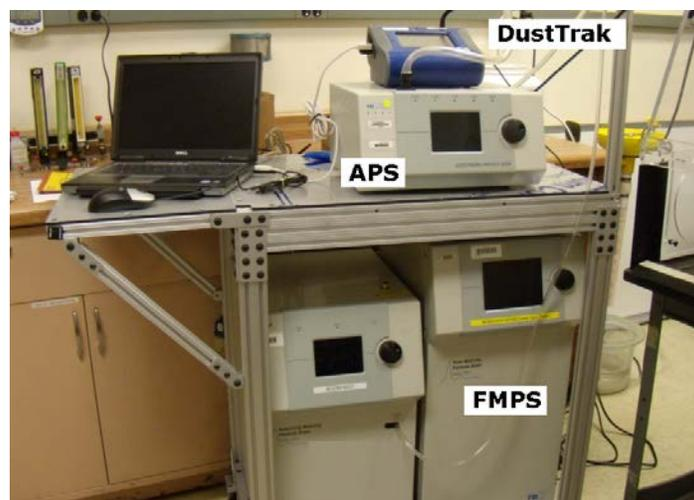
**Figure 3:** Sampling instruments (including the FMPS, APS, and DustTrak) to monitor aerosol emissions.
