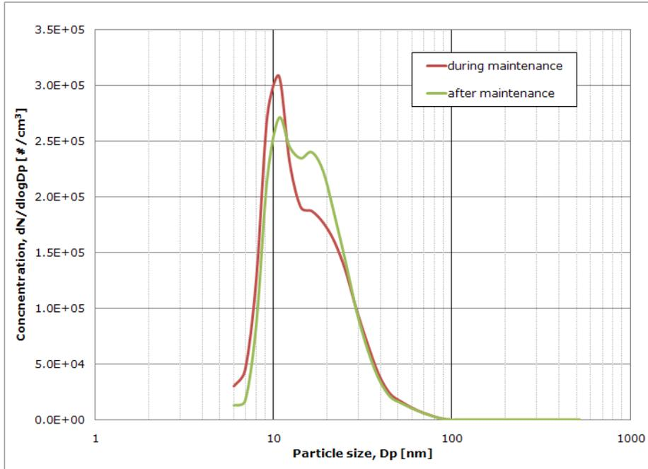
**Figure A-2:** Average size distribution of nanoparticles from the maintenance task performed at the DARPA Furnace monitored by FMPS 2 during process monitoring for Furnace F1 on 09/23/2010. The size distributions after maintenance were calculated by the data between 15:24 (stopping maintenance monitoring of the DARPA Furnace) and 15:26 (before sampling at point 1 inside the F1 enclosure) as referred to in **Figure A-1**.
