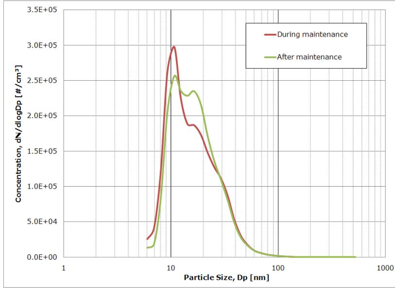
**Figure 10:** Average size distributions from the maintenance tasks performed at the DARPA Furnace monitored by FMPS 1 during process monitoring for Furnace F1 on 09/23/2010. The size distributions after maintenance were calculated with the data collected between 15:22 (stopping maintenance monitoring of the DARPA Furnace) and 15:24 (before sampling at point 1 inside the F1 enclosure) from **Figure 9**.
