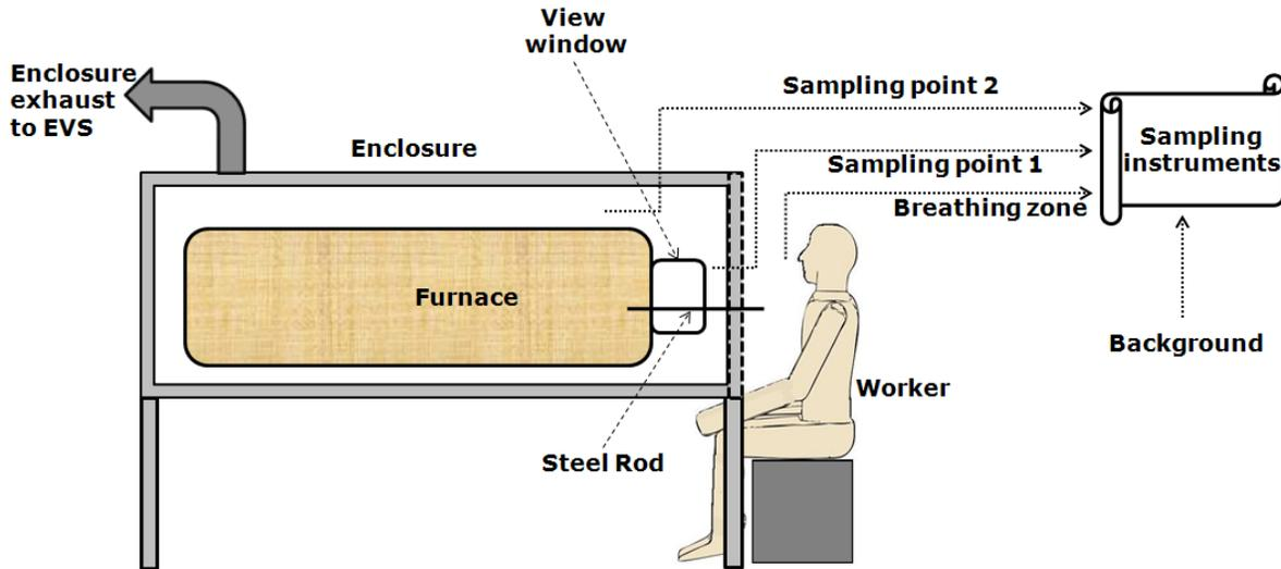
**Figure 4:** Sampling locations during process monitoring. Sampling point 1 was located at the view window to assess the process as a source of nanoparticles. Sampling point 2 was located inside the furnace enclosure to provide information on the source.
