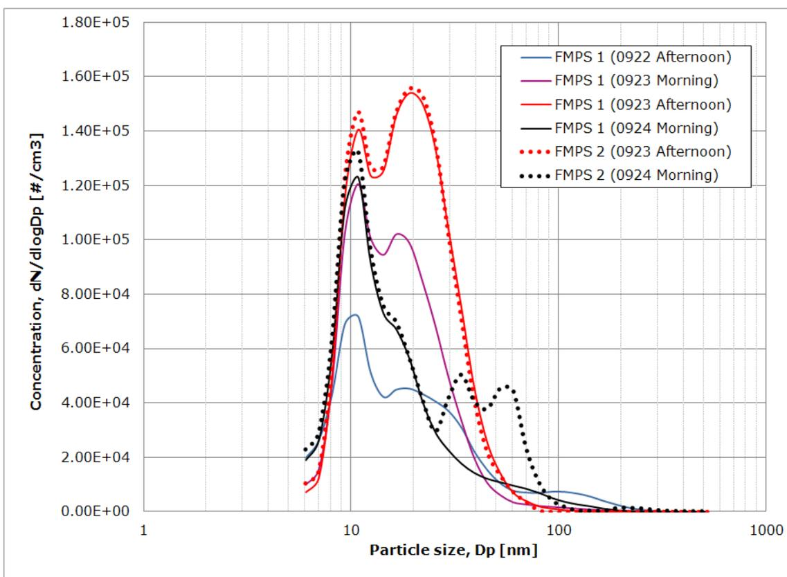
**Figure 6:** Average particle size distributions measured by two FMPS spectrometers for area monitoring on different dates and times.
