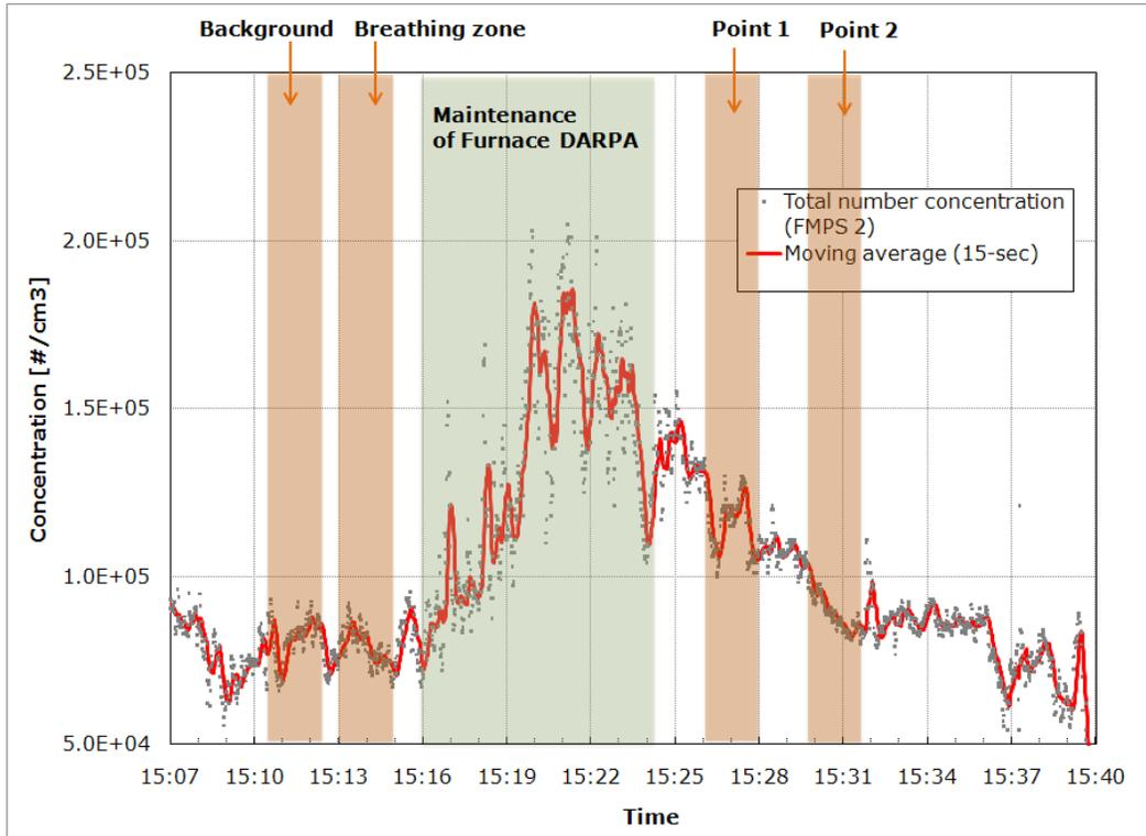
**Figure A-1:** Enclosure efficiency check by FMPS 2 for Furnace 1 on 9/23/2010. The sampling procedures were marked by colored columns to highlight sampling durations and locations. The sampling was halted by moving the sampling ports into the DARPA Furnace to check particle emissions from its 6-minute maintenance. The enclosure test was resumed by finishing two measurements inside Furnace 1.
