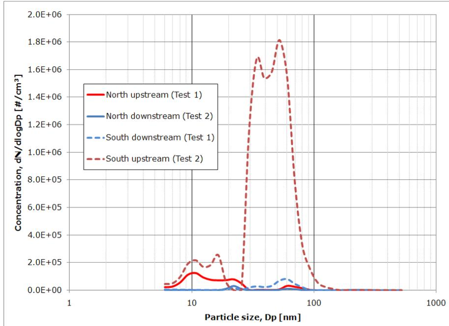
**Figure A-4:** Average size distributions from EVS upstream and downstream measurement by FMPS 2 on 09/24/2010.
