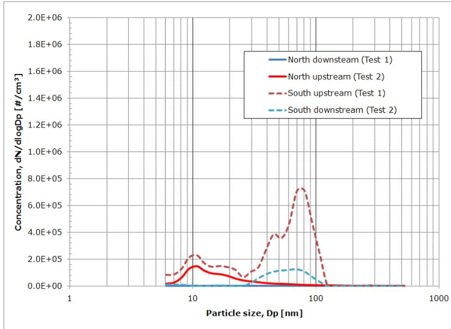
**Figure A-3:** Average size distributions from EVS upstream and downstream measurements by FMPS 1 on 09/24/2010.
