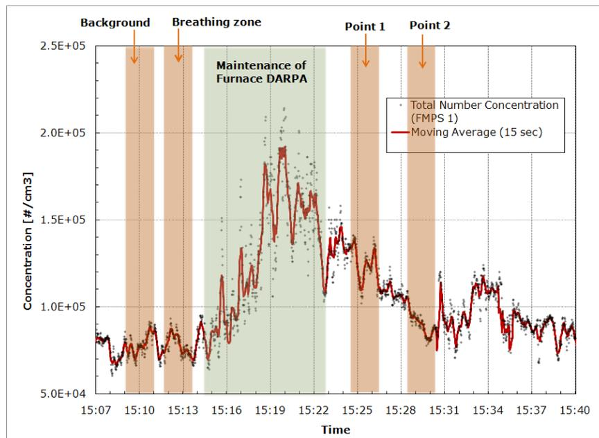
**Figure 9:** Enclosure test by FMPS 1 for Furnace F1 on 09/23/2010. The sampling procedures were marked by colored columns to highlight sampling durations and locations. The sampling was halted by moving the sampling ports into the DARPA Furnace to check particle emissions from its 6-minute maintenance operation. The enclosure test was resumed by finishing two measurements inside Furnace F1.
