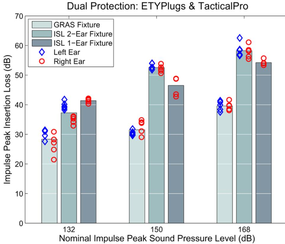
Figure 10: Dual protection Etymotic Research ETYPlugs® Earplug and 3M™ Peltor™ TacticalPro Communications Headset IPIL results. The bars correspond to the average IPIL for each test level as measured on each fixture. The diamonds and circles are the average IPIL values for the left and right ears of each sample.
