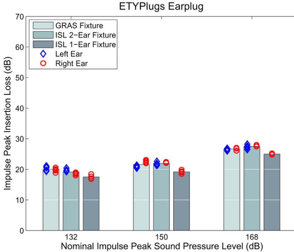
Figure 7: Etymotic Research ETYPlugs® Earplug IPIL results. The bars correspond to the average IPIL for each test level as measured on each fixture. The diamonds and circles are the average IPIL values for the left and right ears of each sample.
