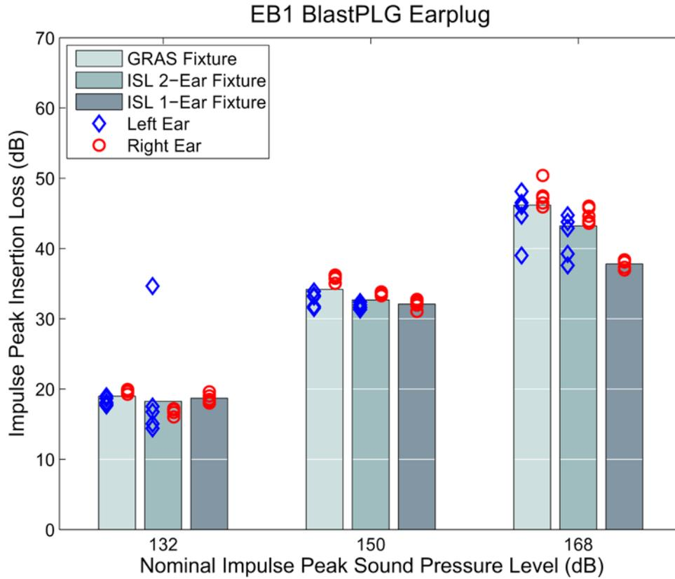
Figure 8: EB1 BlastPLG Earplug IPIL results. The bars correspond to the average IPIL for each test level as measured on each fixture. The diamonds and circles are the average IPIL values for the left and right ears of each sample.
