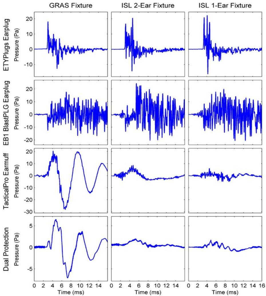
Figure 3: Example occluded waveforms measured at the 132-dB impulse level for the dual-ear GRAS, dual-ear ISL and single-ear ISL fixtures using ETYPlugs earplug, EB1 BlastPLG earplug, Peltor TacticalPro earmuff and Dual Protection with TacticalPro earmuff combined with ETYPlugs earplug.
