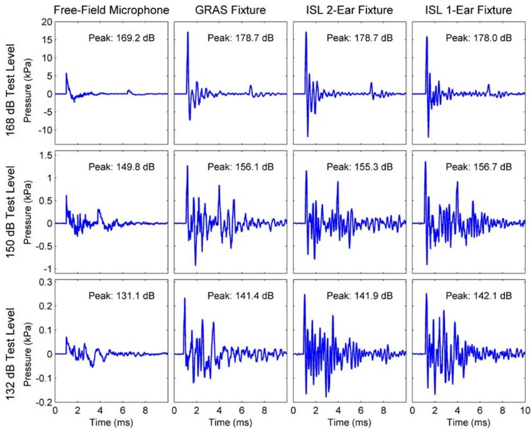
Figure 2: Example unoccluded waveforms measured from the field microphones and acoustic test fixtures for the 132-dB, 150-dB and 168-dB impulse levels. The free-field microphones were fixed in the same location while the three fixtures were rotated through all three positions.
