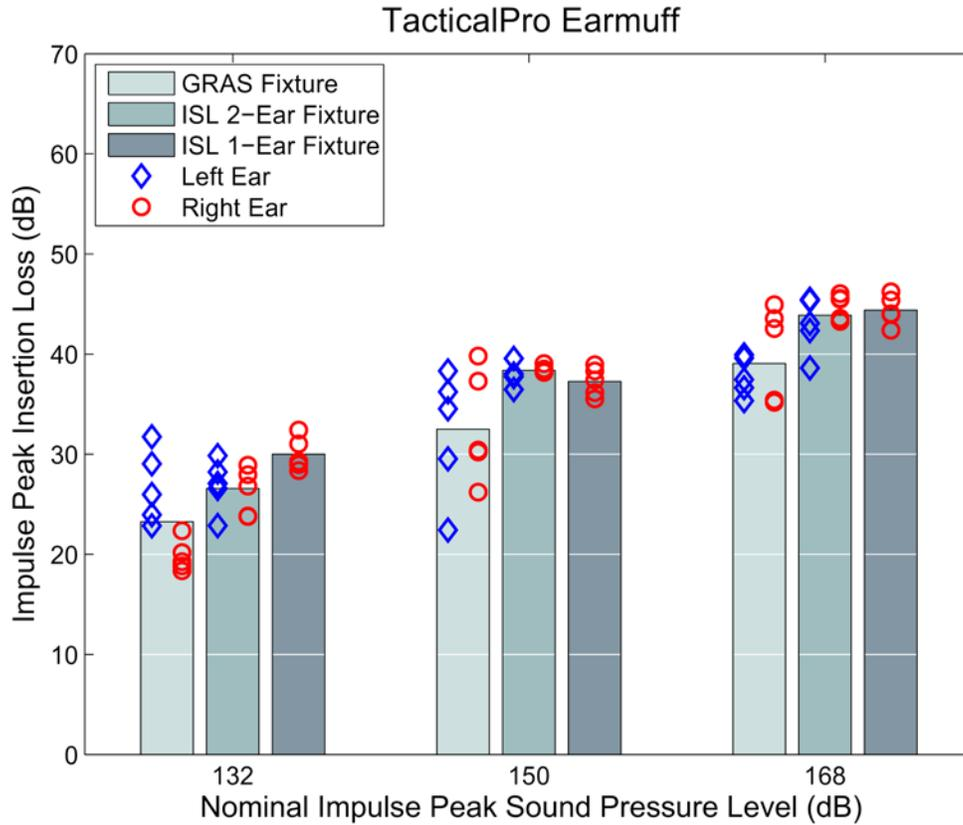
Figure 9: 3M™ Peltor™ TacticalPro Communications Headset (tested with electronics on and set to unity gain) IPIL results. The bars correspond to the average IPIL for each test level as measured on each fixture. The diamonds and circles are the average IPIL values for the left and right ears of each sample.
