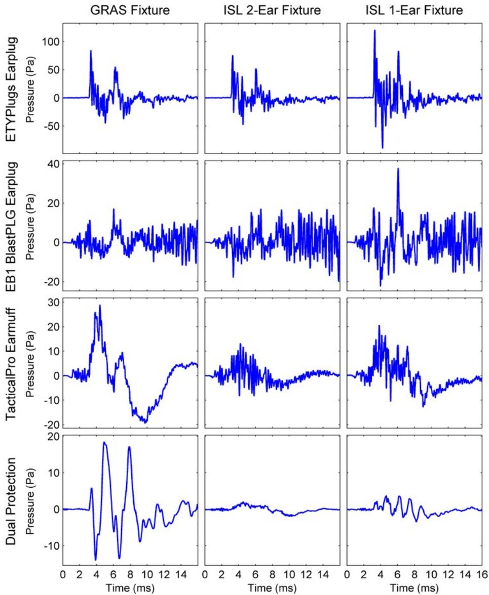
Figure 4: Example occluded waveforms measured at the 150-dB impulse level for the dual-ear GRAS, dual-ear ISL and single-ear ISL fixtures using ETYPlugs earplug, EB1 BlastPLG earplug, Peltor TacticalPro earmuff and Dual Protection with TacticalPro earmuff combined with ETYPlugs earplug.
