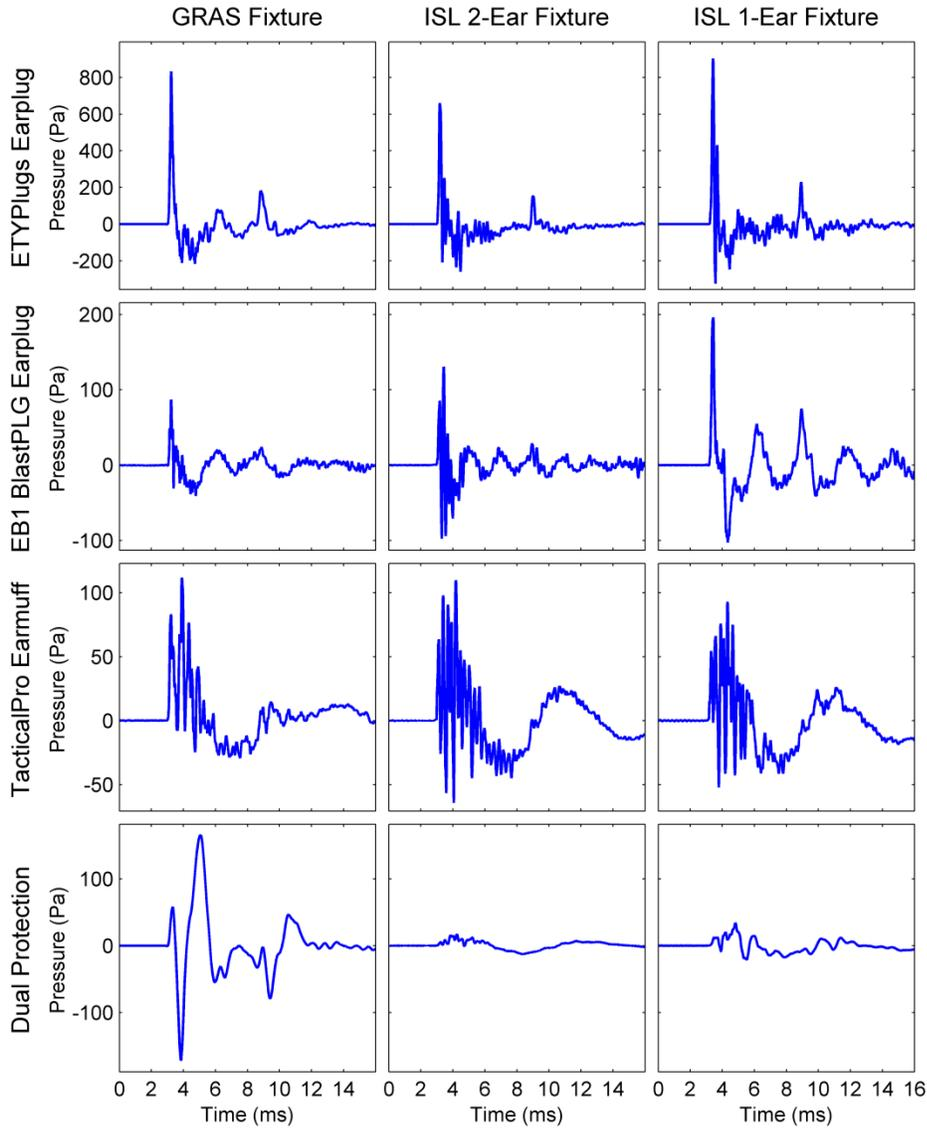
Figure 5: Example occluded waveforms measured at the 168-dB impulse level for the dual-ear GRAS, dual-ear ISL and single-ear ISL fixtures using ETYPlugs earplug, EB1 BlastPLG earplug, Peltor TacticalPro earmuff and Dual Protection with TacticalPro earmuff combined with ETYPlugs earplug.
