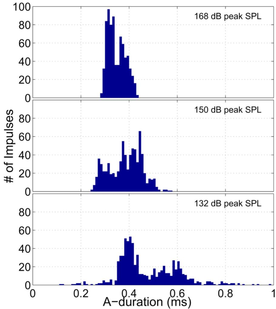
Figure 6 A-duration data for the impulses produced by .223 caliber Colt AR-15 rifle were measured with the free-field microphones. The A-durations varied between 0.24 to 0.45 ms at the 168-dB impulse level, 0.24 to 0.58 ms at the 150-dB impulse level and 0.11 to 0.98 ms at the 132-dB impulse level.
