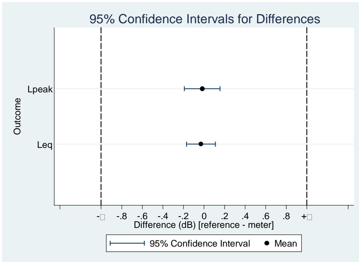
**Figure 10. Mean and confidence intervals for the differences between the reference system and the new meter**
