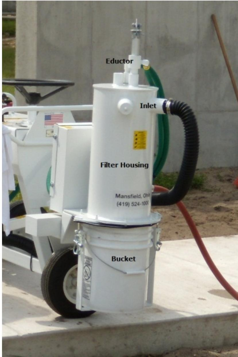
Figure 4 - Dust Collector (Inlet, Eductor, Bucket and Filter Housing Labeled)
