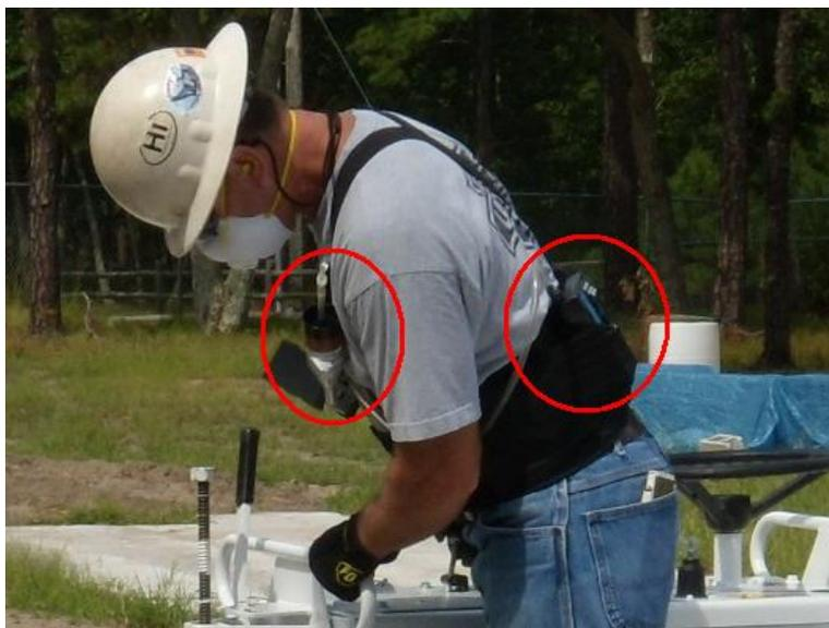
**Figure 2 – Laborer Wearing Pump and Cyclone (Circled)**
