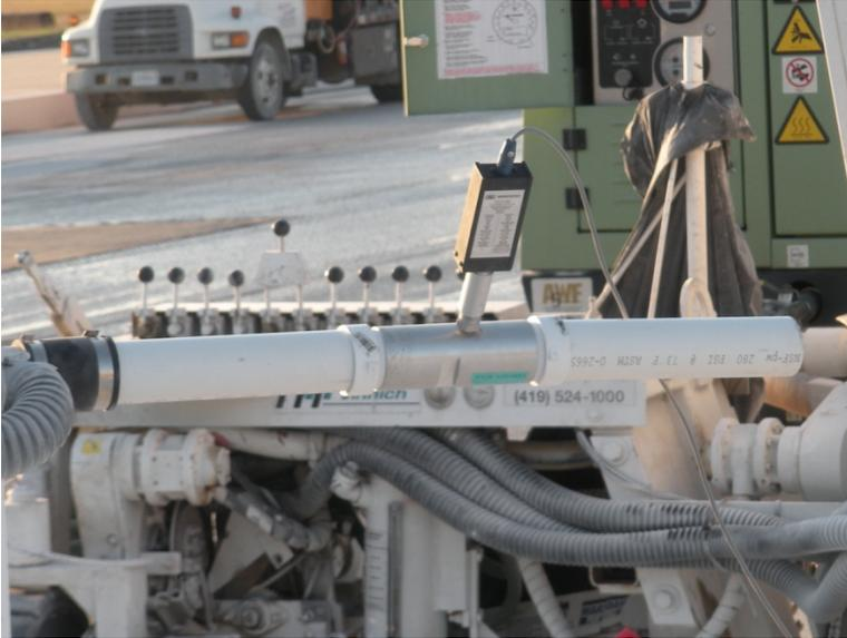
Figure 5 - Air Flow Measurement Device on Company-Owned Drill
