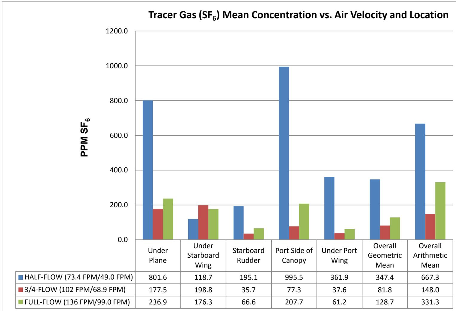
**Figure 12. Time-averaged concentrations of SF<sub>6</sub> by measurement location and ventilation system status. Values at the five locations are geometric means for trials of three source configurations. Overall geometric and arithmetic means were calculated over the (5 x 3 = 15) individual observations.**
