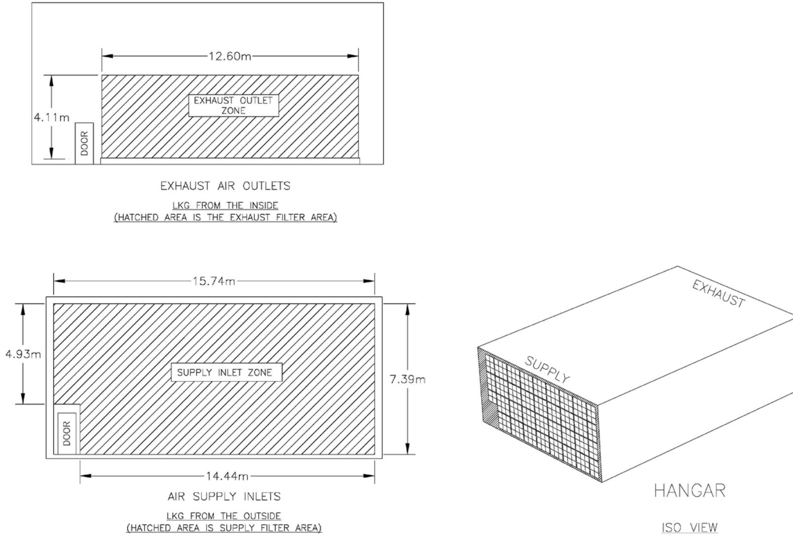
Figure 1. Drawing showing filter area of Bay 6, Building 465, Fleet Readiness Center Southwest, San Diego, CA.
