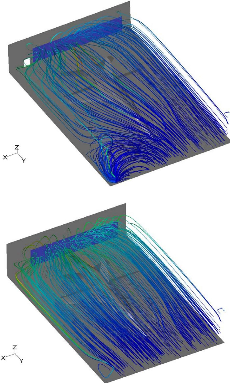
**Figure B-2.** Visualized flow lines colored by residence time for the unbalanced 108 fpm supply-65.0 fpm exhaust case (top image) and the balanced 65.0 fpm case (bottom image).
