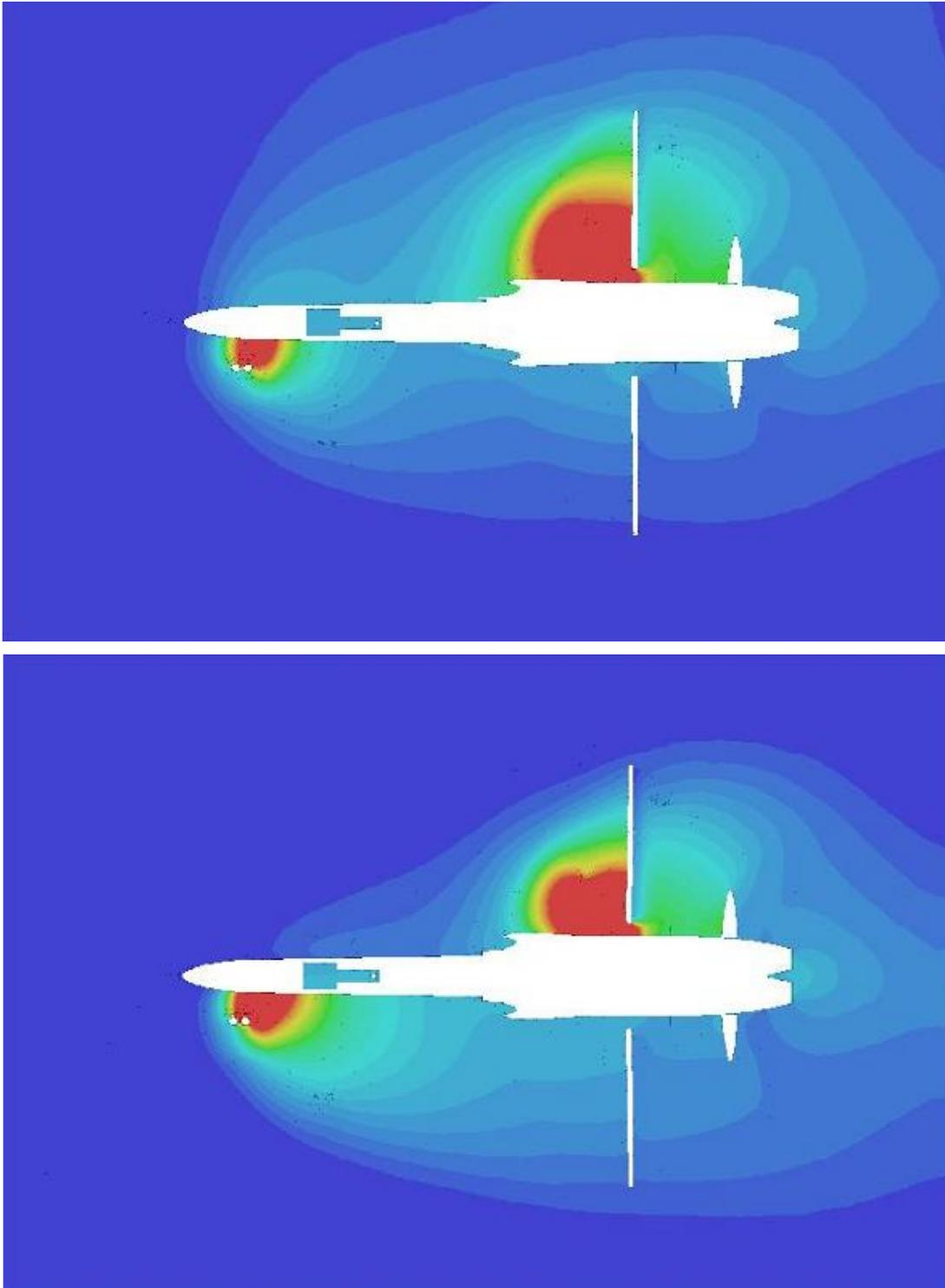
**Figure B-1.** Contours of MIBK concentration at breathing zone height for the unbalanced 108 fpm supply-65.0 fpm exhaust (top image) and the balanced 65.0 fpm (bottom image) cases.
