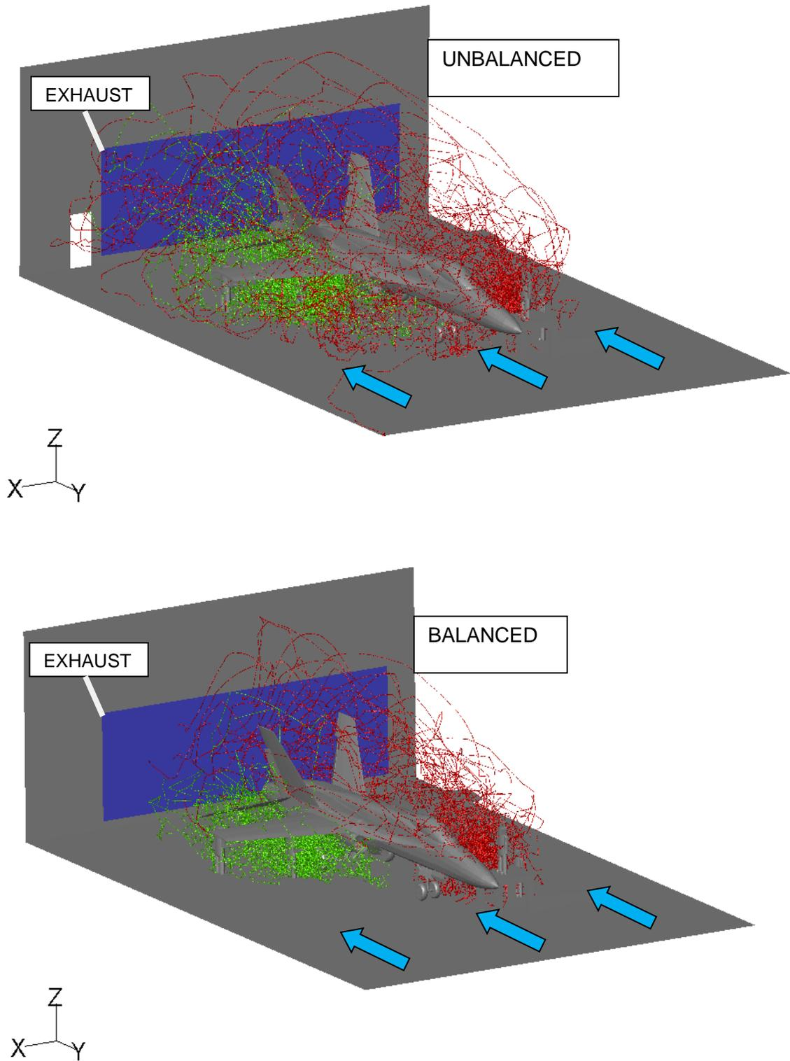
**Figure 11.** Particle tracks for the unbalanced 108 fpm supply – 65.0 fpm exhaust case (top image) and the balanced 65.0 fpm case (bottom image). The balanced case shows less particle dispersion.
