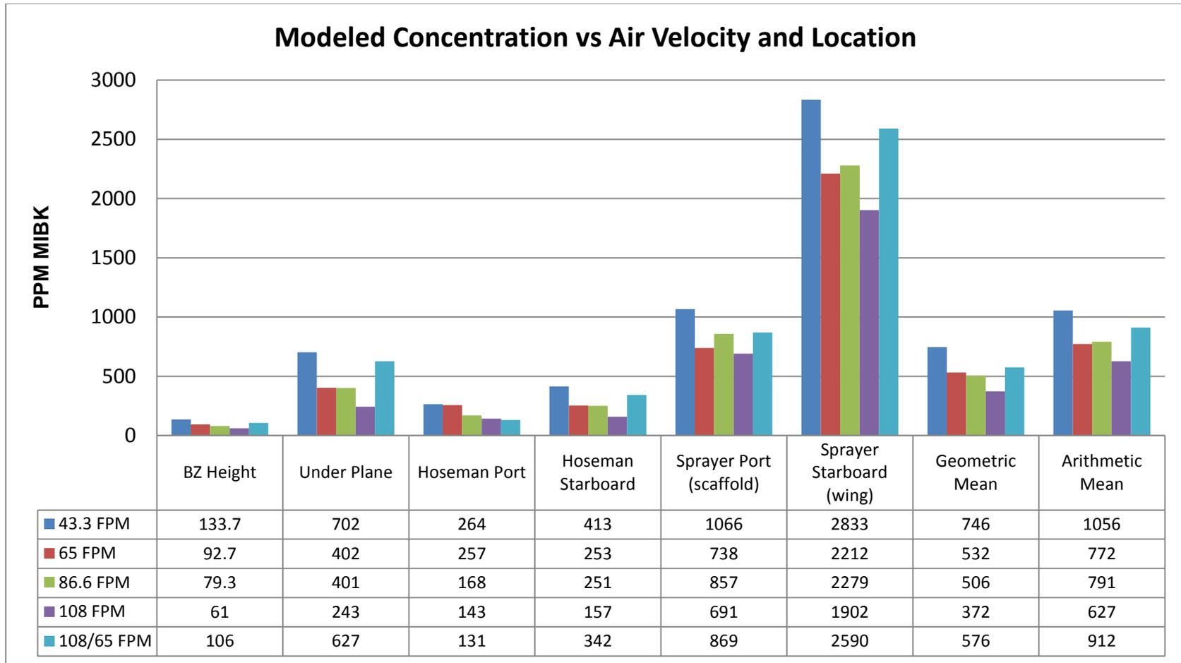
**Figure 9. Concentrations of a gas with the properties of MIBK calculated using CFD, for various air velocities and observed worker locations. 108/65 fpm indicates the unbalanced condition of 108 fpm of supply and 65 fpm of exhaust.**
