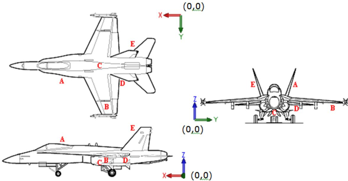
Figure 7: Approximate locations of the five MIRAN<sup>®</sup> Sapphires around the F/A-18C/D Hornet during the first release scenario. Source:
