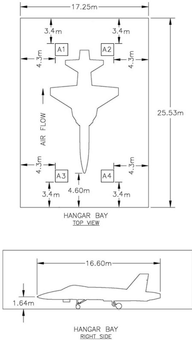
**Figure 2. Drawing showing interior of bay, F/A-18C/D Hornet, and area sample locations (A1 – A4). Bay 6, Building 465, Fleet Readiness Center Southwest, San Diego, CA.**
