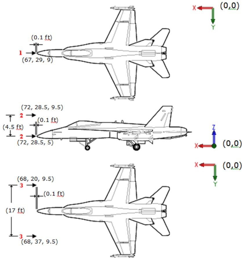
Figure 6: Source locations for the release of SF<sub>6</sub> near the front of the F/A-18C/D Hornet. Source: <http://www.boeing.com/defense-space/military/fa18/fa18cd3v.htm>
