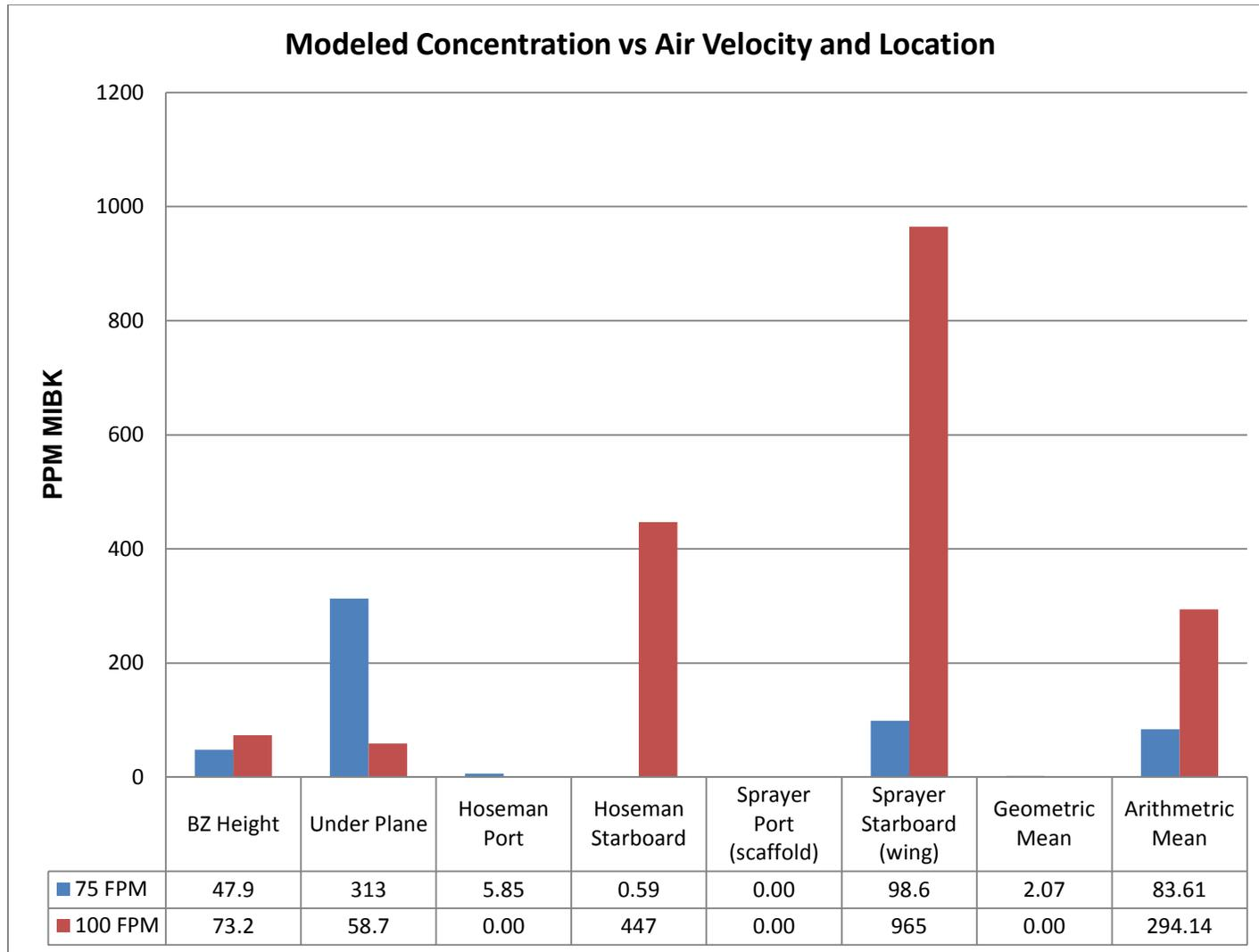
Figure 10. CFD results at 75 fpm and 100 fpm using the RNG k-epsilon turbulence model and a convergence criterion of  $10^{-4}$  for the normalized residuals.
