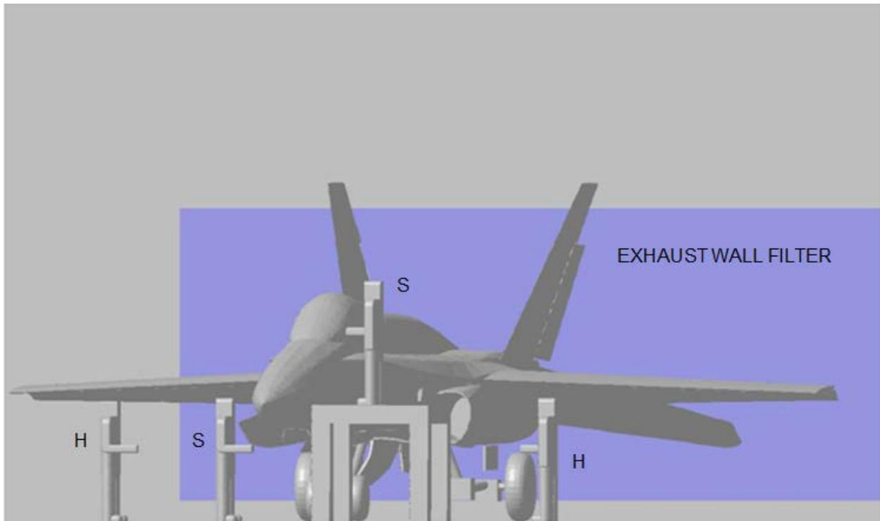
**Figure 5. Geometry of simulated workers, exhaust wall filter, and F/A-18C/D Aircraft. Hosemen (H) are further from the aircraft and further downwind than sprayers. The contaminant source is located at the end of the sprayers' (S) right arms. One sprayer is on a scaffold.**
