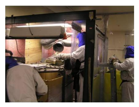
Figure VII – Electron Gun Removal in Glass Breaking Operation
