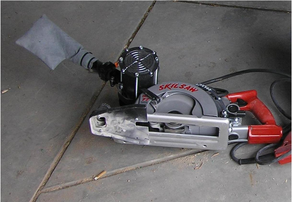
Figure 1. Saw with aftermarket local exhaust ventilation.
