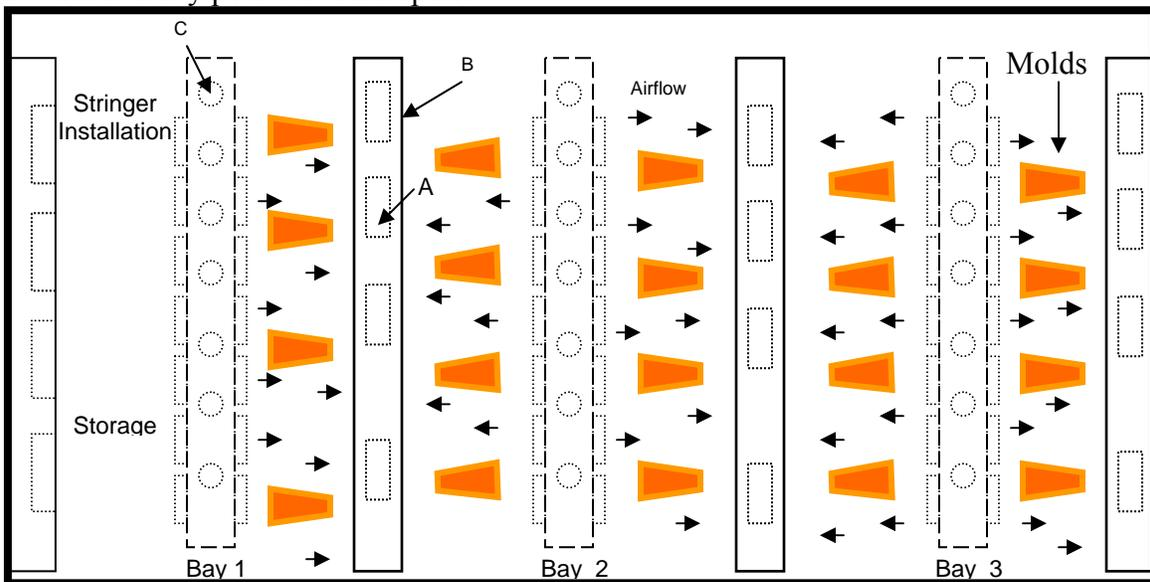
**Figure 1:** Plan View of Controlled-flow Ventilation installed by Frees Inc.
