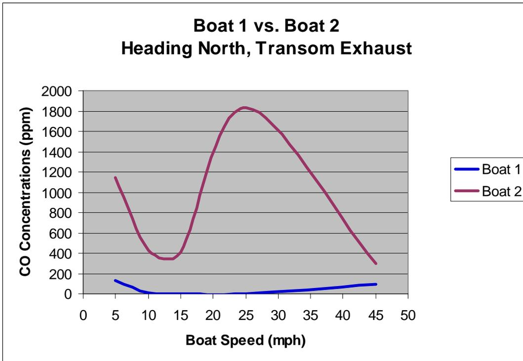
**Figure 8: Ferret Data Measured Directly Into the Exhaust Opening**
