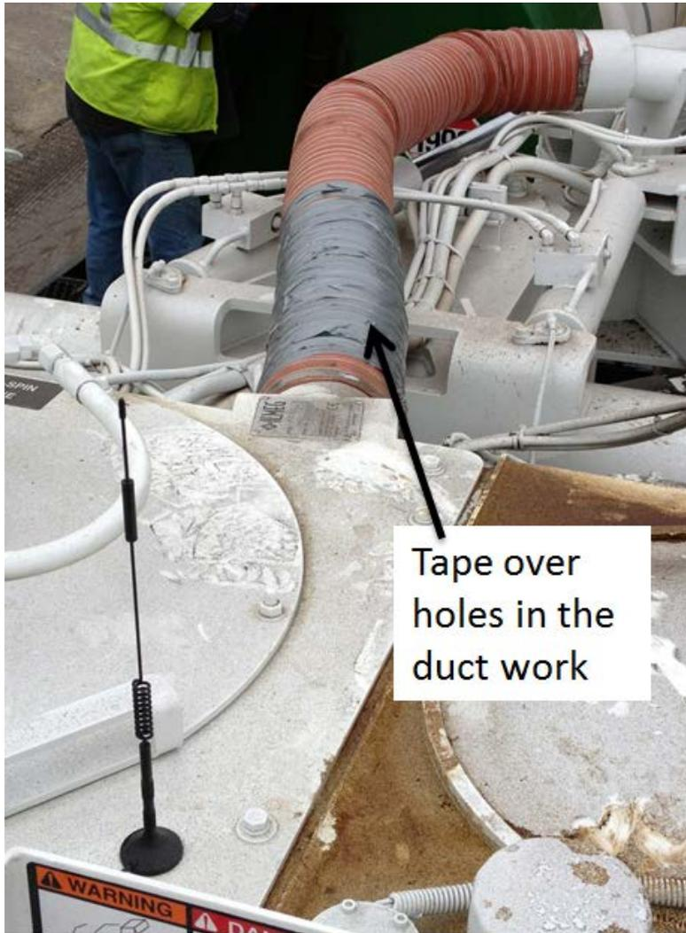
Figure 2: Tape over duct work near the fan outlet
