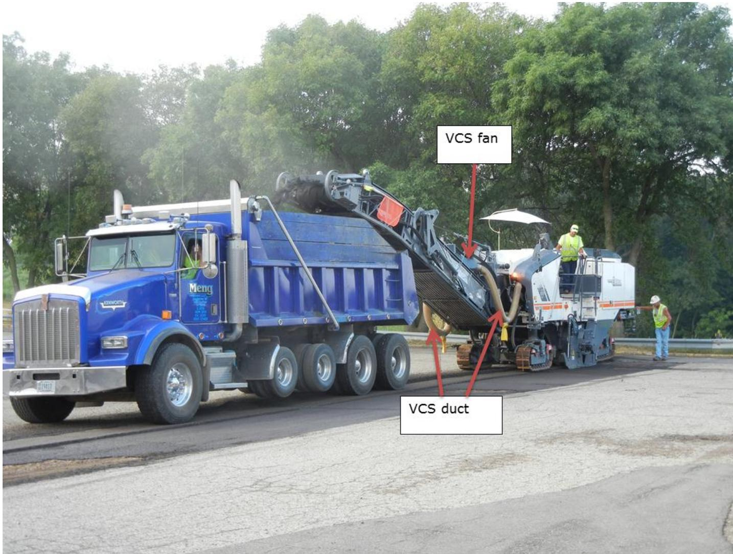
Figure 1: Wirtgen milling machine with VCS
