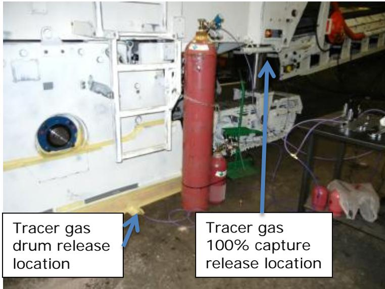
Figure 3: tracer gas injection locations
