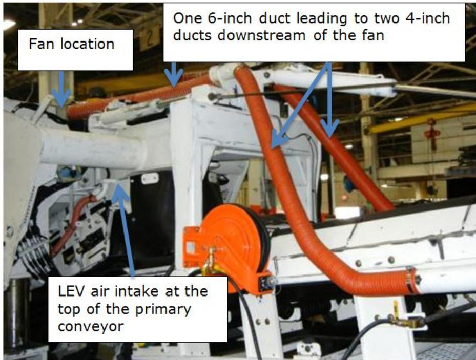
Figure 6: LEV air intake at the top of the primary conveyor.
