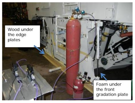
Figure 1: Wood, tape, and foam used to fill in gaps.
