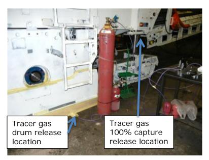
Figure 3: tracer gas injection locations
