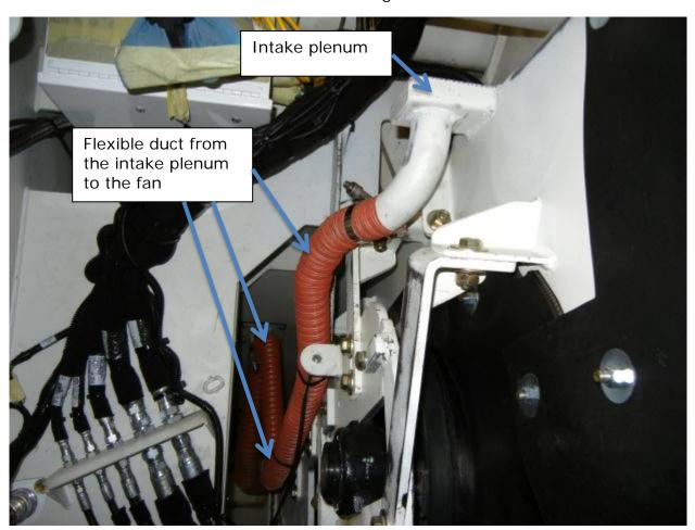
Figure 7: Flexible duct on the suction side of the fan
