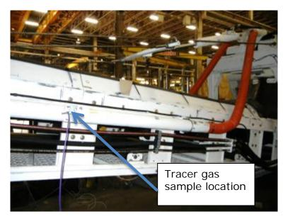
Figure 4: Tracer gas sampling location
