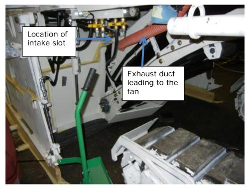
Figure 5: LEV air intake at the bottom of the primary conveyor
