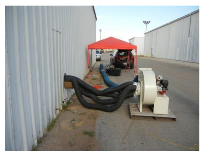
Figure 2: Fan and ductwork for prototype LEV testing.
