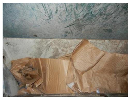
Figure 7: Obstruction stuffed in the outlet of the primary conveyor.
