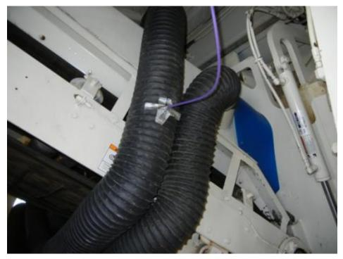
Figure 5: LEV exhaust locations along the left side of the primary conveyor.
