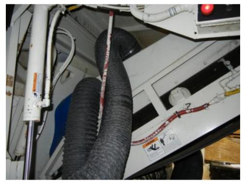
Figure 6: LEV exhaust locations along the right side of the primary conveyor.
