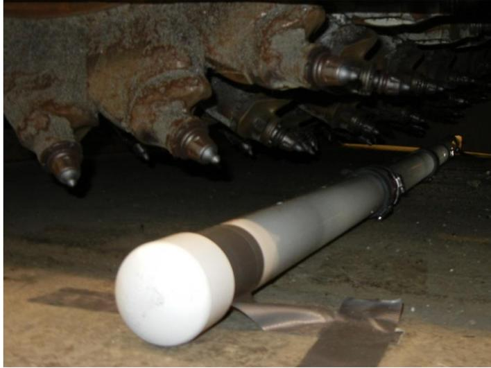
**Figure 3: Smoke test pipe placement**
