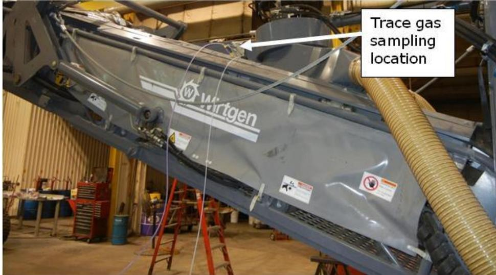
**Figure 6: Sampling probe placement**
