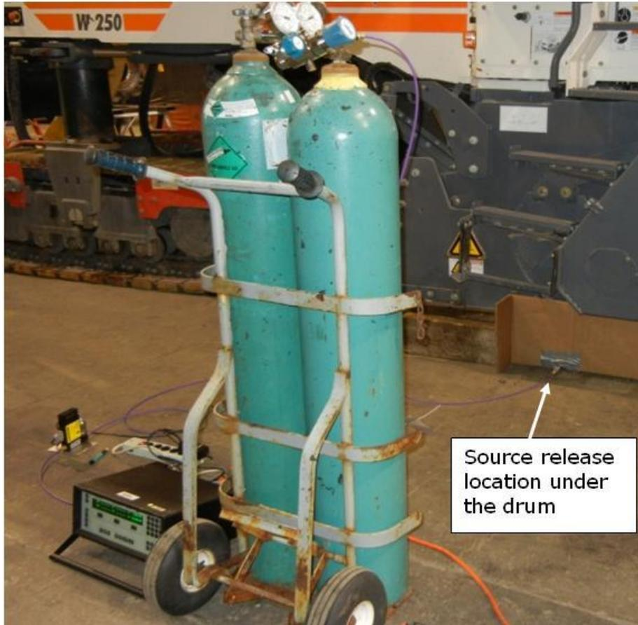
**Figure 5: Tracer gas source**
