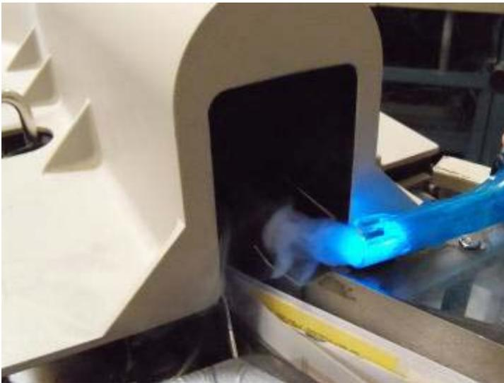
**Figure 23: Smoke entering the BDS hood near the upstream face and location G**
