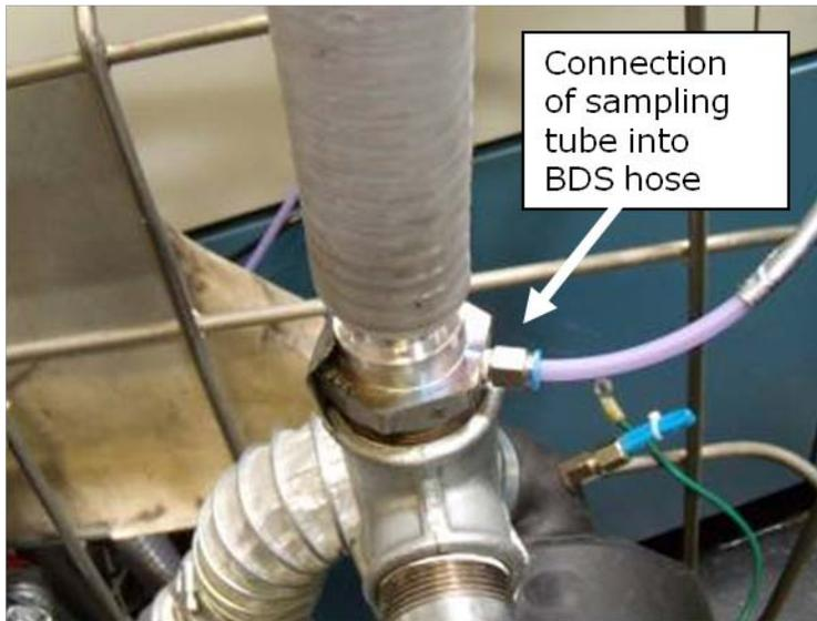
**Figure 14: Connection of sampling tube to the BDS hose**
