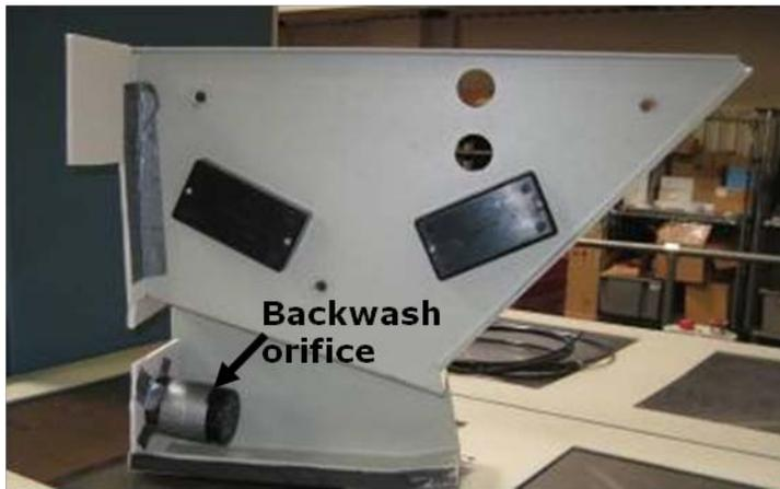
**Figure 8: Low Flow Backwash Orifice added to the Prototype AFCS 200 machine**
