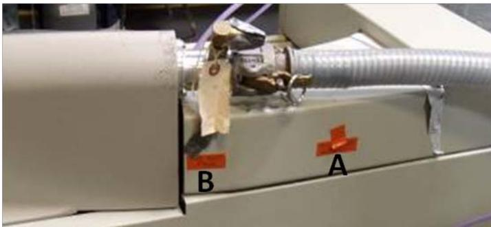
**Figure 16: Tracer gas release locations A and B for the BDS hood**
