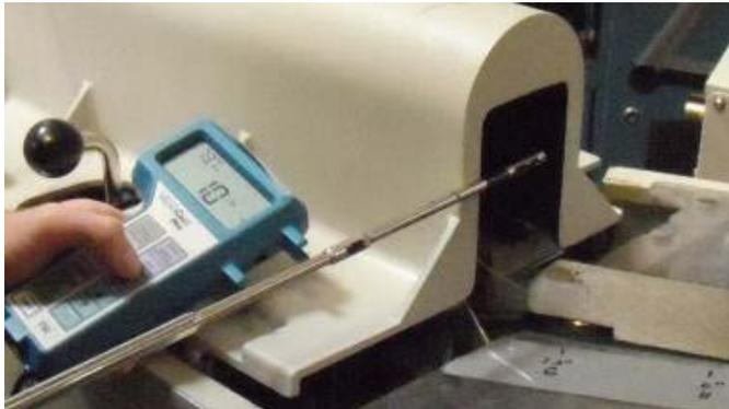
**Figure 19: Hot wire anemometer used to measure capture velocity**
