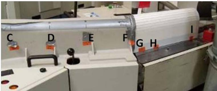
**Figure 15: Tracer gas release locations C through I for the BDS hood**
