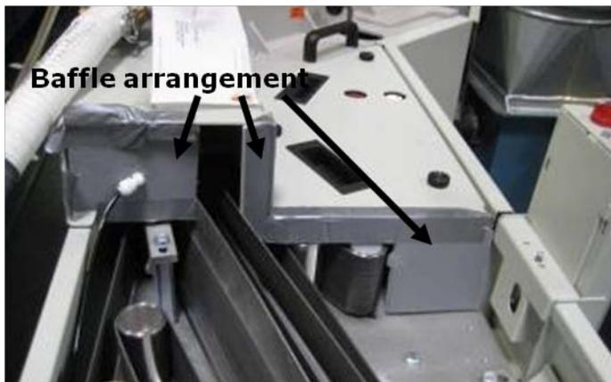
Figure 6: Baffle Arrangement on the Prototype AFCS 200 machine 1<sup>st</sup> cover
