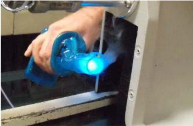
**Figure 22: Smoke entering the downstream face of the BDS hood when the flow of mail was interrupted.**
