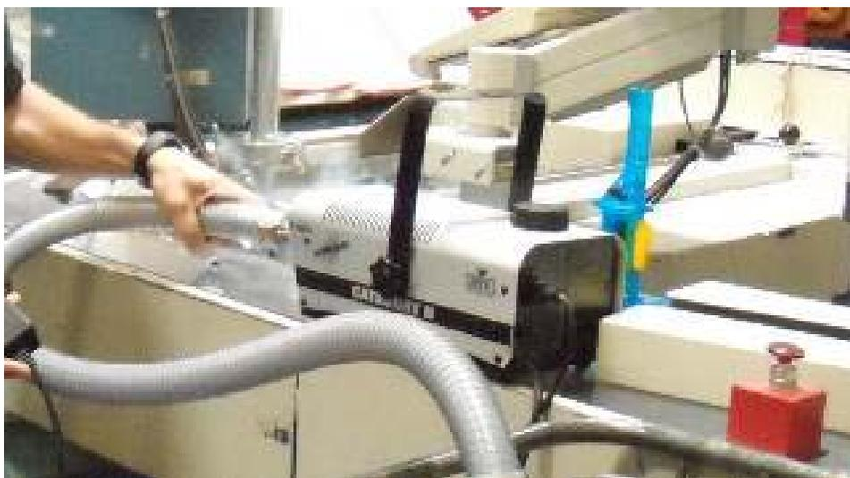
**Figure 18: Fog machine for larger quantity smoke release**
