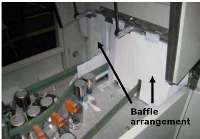
Figure 7: Baffle Arrangement on the Prototype AFCS 200 machine 2<sup>nd</sup> cover
