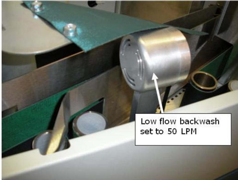
**Figure 3: Low-flow backwash orifice set to 50 ALPM**
