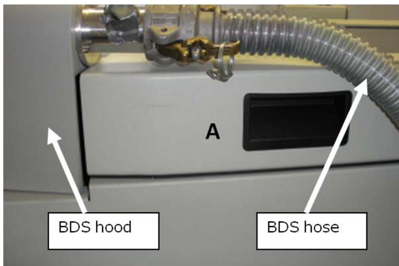
**Figure 7: Tracer gas location A for the BDS hood of the AFCS 200**
