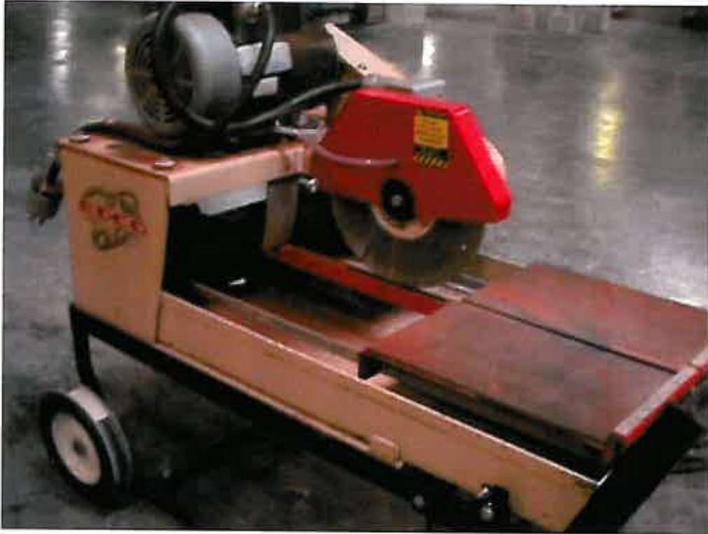
Figure 11. EDCO GMS10 brick saw with an exhaust take-off. This unit was operated with an electric motor in place of a gas motor. The exhaust slot is 6.625 inches long and 5/16 inches wide. The exhaust channel under the blade is 1 inch square.
