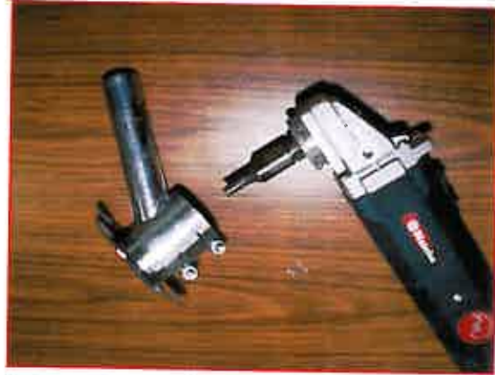
B. MORTAR RAKE MOUNTED ON GRINDER
