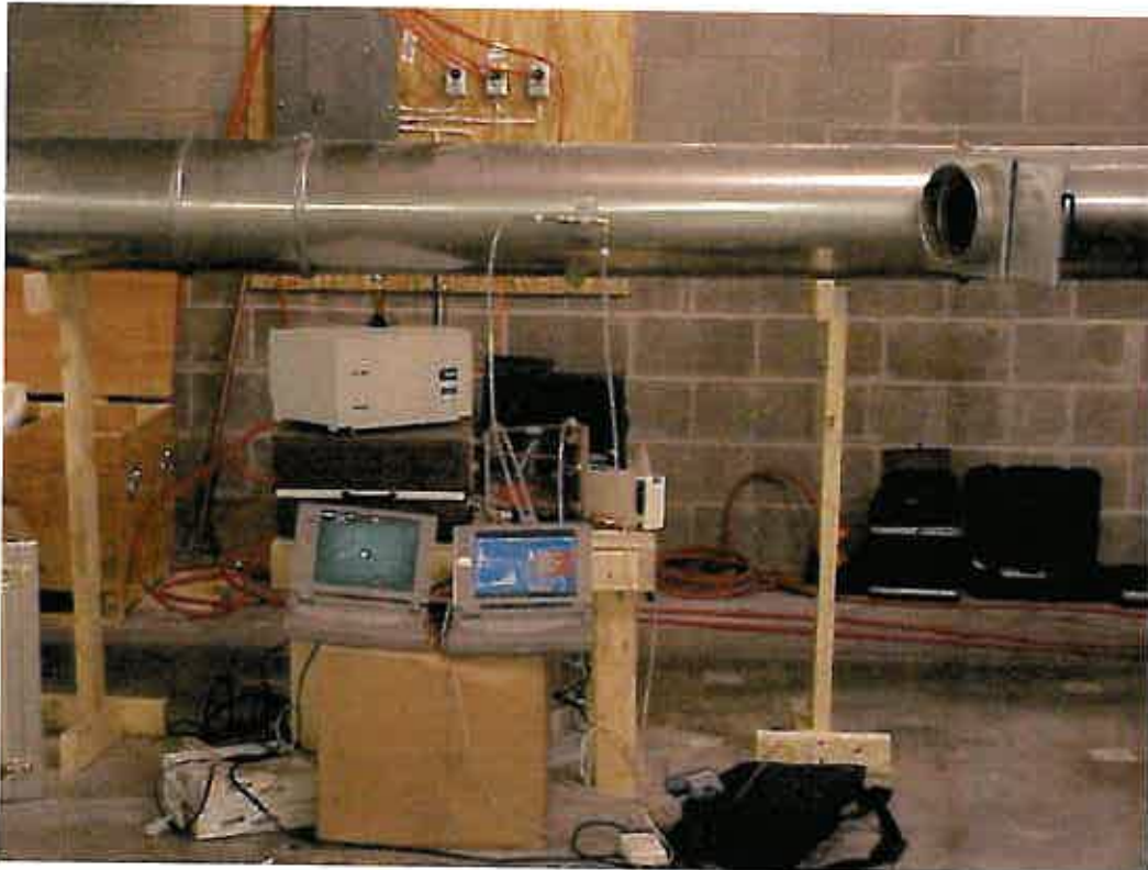
Figure 6 Photograph of instruments and isokinetic sampling location. The blast gate position was adjusted to obtain a 1.95 inches of water across the delta tube.
