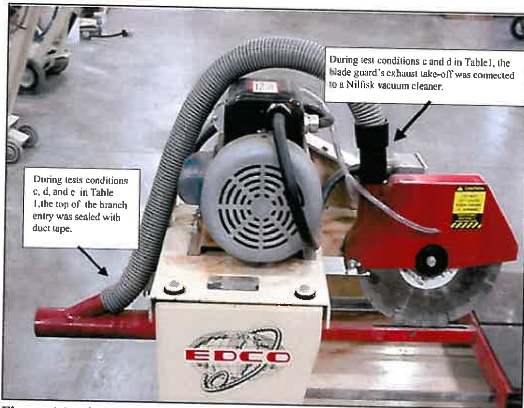
Figure 14. GMS10 masonry saw modified to have an exhaust take-off on the blade guard.
