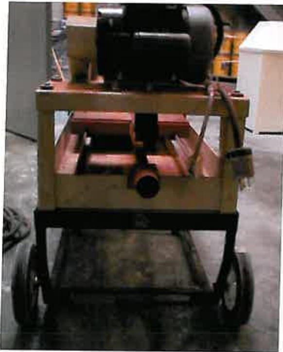
Figure 13 A 2-inch diameter exhaust port for the EDCO brick saw. When brick cutting is done without ventilation, the dust naturally flows out this exhaust take-off.
