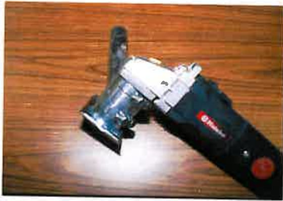
A. MORTAR RAKE, SHROUD ON A RIGHT ANGLE GRINDER
