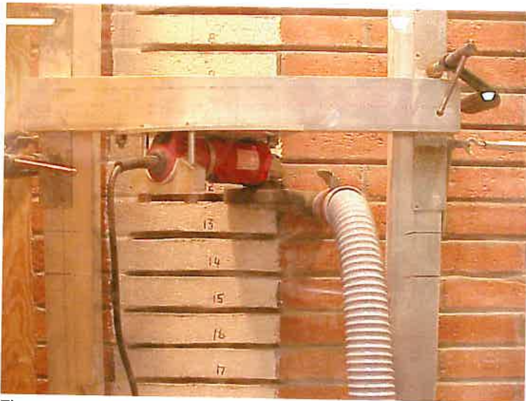
Figure 5. Grinder mounted on a frame. The grinder moves to the right.
