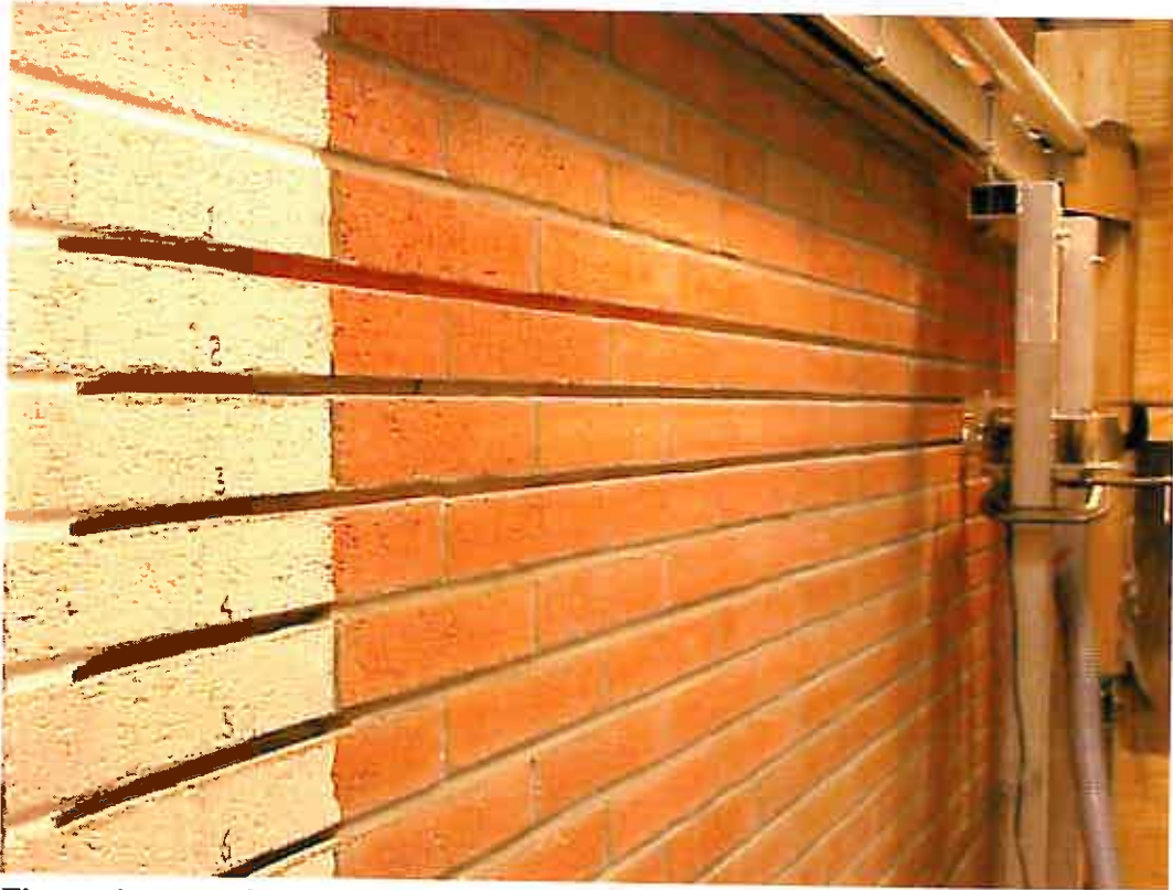
Figure 4. The frame moving down the wall toward the air cleaner.
