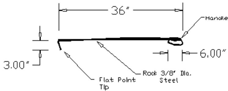
Figure 13. Sorting Parts Hook
