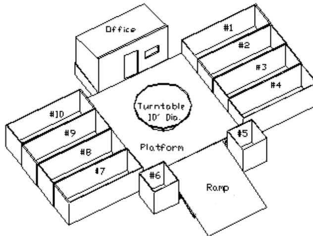
Figure 12. Elevated Rotating Sorting Table
