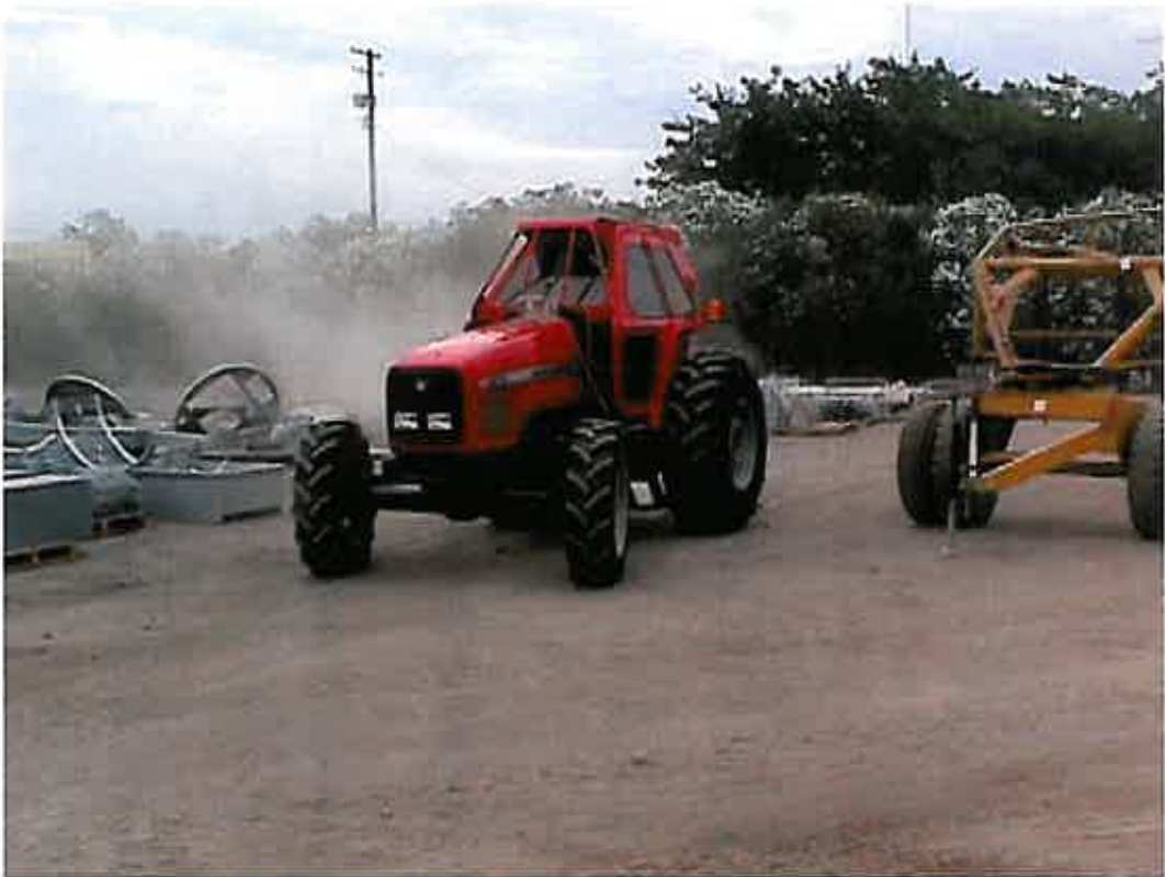
Figure 4. Tractor being driven during the mobile test. This test was conducted on the unpaved surfaces in the Nelson Manufacturing Company back lot.
