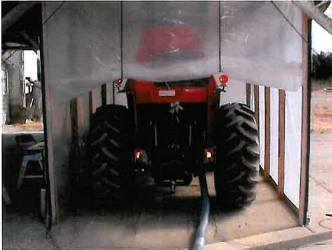
Figure 7. Tractor in the test enclosure for the stationary testing. A roll of polyethylene was raised or lowered in an effort to control the incense aerosol concentration in the enclosure. Note, the flexible metal duct was used to transport engine exhaust out of the enclosure.
