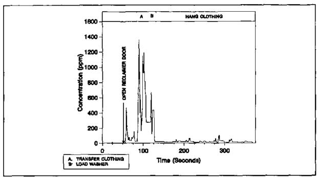
Figure 7 Operator exposure during transfer, loading washer and hanging clothing
