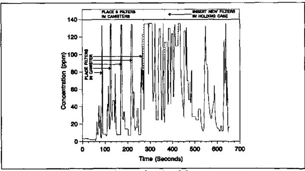
Figure 10 Worker exposure during changing filters
