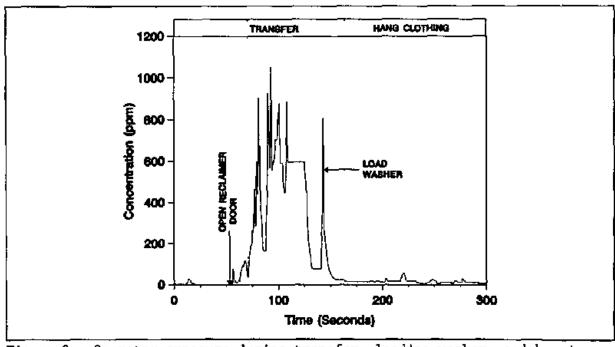
Figure 8 Operator exposure during transfer, loading washer, and hanging clothing
