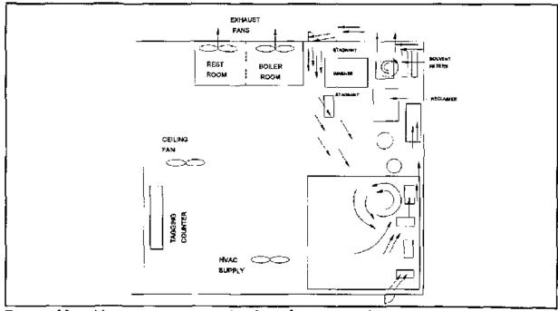
Figure 12 Air currents near the dry-cleaning machines
