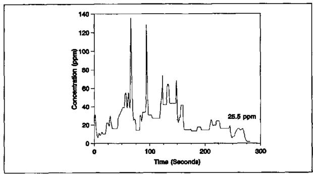
Figure 9 Operator exposure during cleaning lint traps
