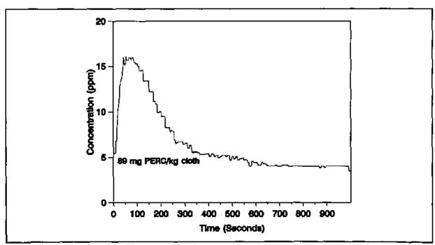
Figure 11 Typical off-gassing of test swatch
