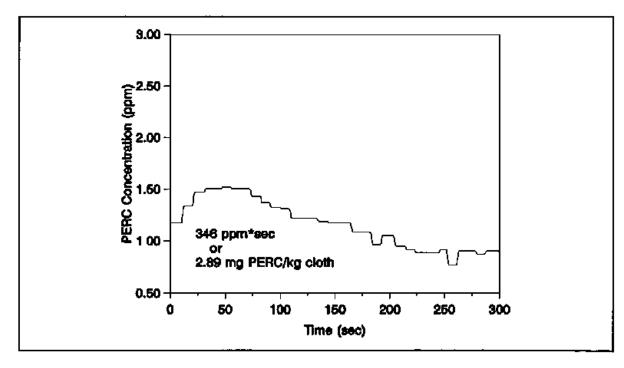
Figure 11 Typical off-gassing of swatch from 36 lb machine
