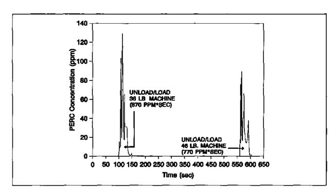
Figure 7 Operator exposure during unloading/loading
