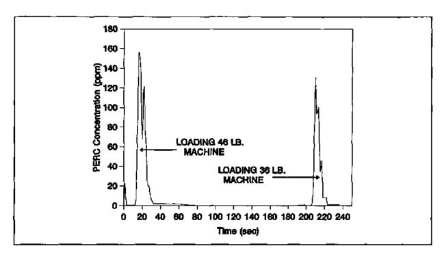
Figure 5 Operator exposure during first cycle of day
