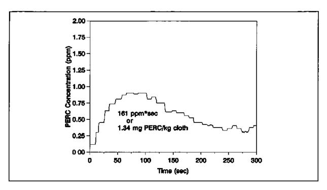
Figure 10 Typical off-gassing of swatch from 46 lb machine
