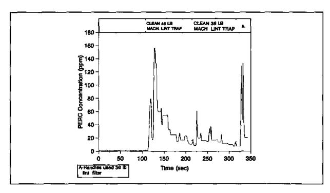
Figure 9 Operator exposure while cleaning lint traps
