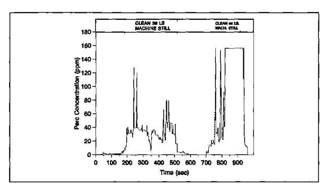
Figure 8 Operator exposure while cleaning the stills
