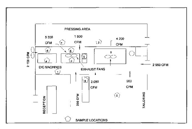
Figure 12 Airflow Balance In/Out of Dry-cleaning Room
