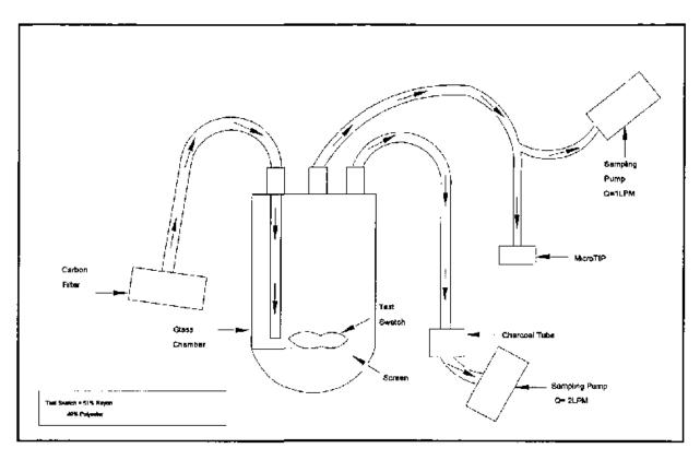
Figure 4 Apparatus for measuring off-gassing of garments and machine recovery
