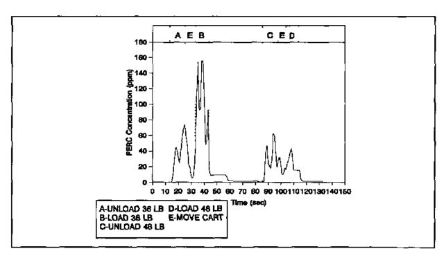
Figure 6 Operator exposure during unloading/loading
