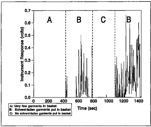
Figure 4 Real Time Solvent Concentrations Over Basket
