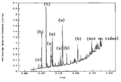
Graph Bl 8/24/94 This data was not coded as it was collected using the NiCad battery which caused the gradual rise in exposure Total sampling time was 55 minutes
