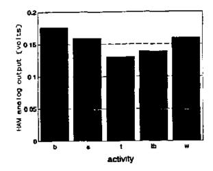
Figure 5 The response of the HAM does not appear to vary much with the activity HAM analog outputs shown are the anthmetic averages for each activity
