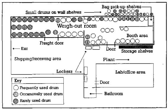
Figure 2 Dye weigh-out room at Multi Color Industries after installation of booth
