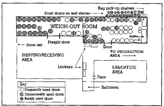
Figure 1 Dye weighout room at Multi Color Industries
