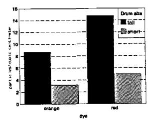
Figure 12 Effect of drum height upon the concentration of particles  $> 0.3 \mu m$  for two dyes
