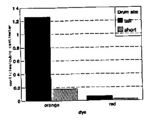
Figure 11 Effect of drum height upon concentration of particles > 3.0  $\mu$ m appears to vary with the dye tested
