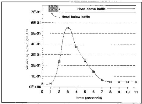
Figure 11 There is a delay between act of placing the head below the baffle and the transitory increase in HAM analog output
