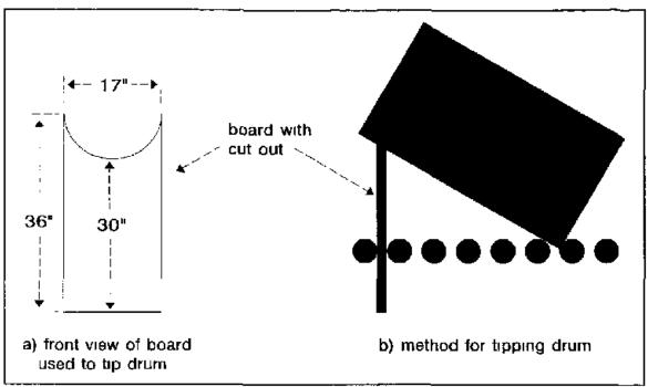
Figure 7 Schematic illustration of cut-out board used to tip drum
