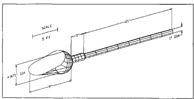
Figure 6 Schematic of long-handle scoop used to remove material from the bottom of a drum
