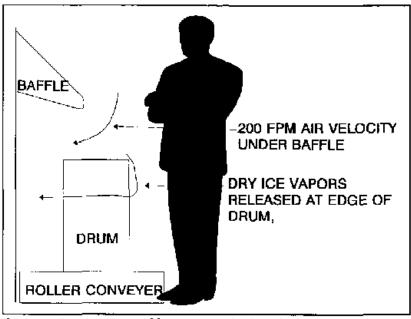
Figure 5 Air flow around the drum
