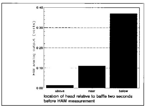
Figure 10 Placing head below baffle increases dust exposure (Data collected during second sampling session )
