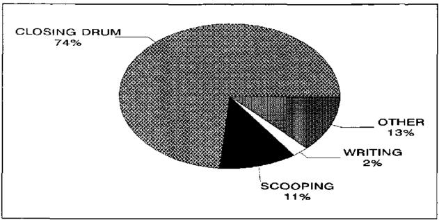
Figure 8 Effect of activity upon percent of total exposure to particles greater that 3  $\mu$ m as measured by the optical particle counter during second sampling session
