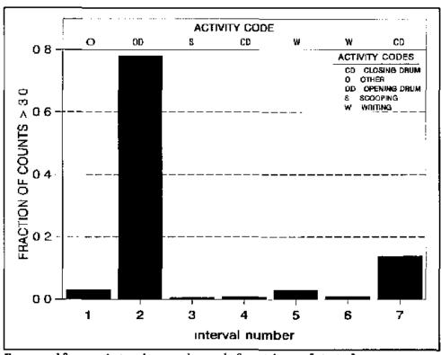
Figure 12 Activity code and fraction of total exposure to particles greater than 3  $\mu$ m measured by the optical particle counter during the third sampling session
