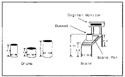
Figure 3. Dimensions of Scale and Drums Used in Booths 1 and 2
