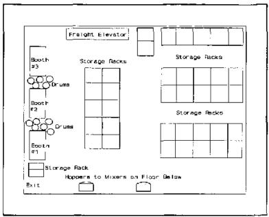
Figure 1. Plant Layout in Weigh-out Area
