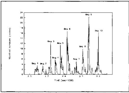
Figure 4 Relative Worker Exposure during Manual Weigh-Out Operation
