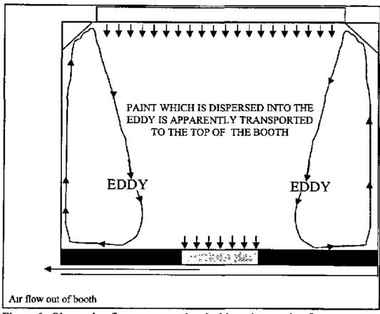
Figure 6 Observed airflow patterns in booth Note, the actual airflow patterns appeared to be more three dimensional
