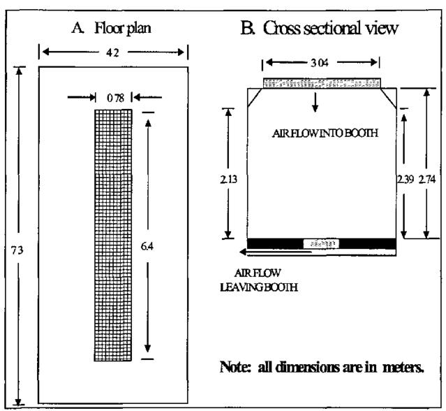
Figure 5 Schematic drawing of the spray painting booth
