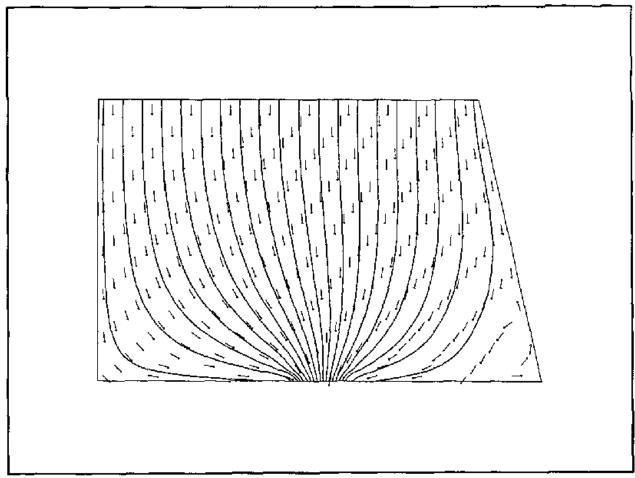
Figure 8 Predicted airflow patterns in a hypothetical booth. On the right side of the booth, the cornice was replaced with a slanted wall. On the left side of the booth, the cornice was eliminated and the air filter in the ceiling was extended to the wall. The solid lines indicate the path of particles released at the ceiling and the arrows indicate the direction of the air flow.
