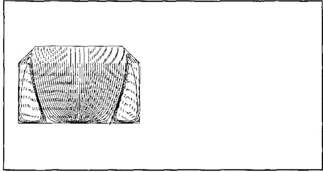
Figure 7 Predicted airflow patterns in existing downdraft booth. The arrows indicate direction of air flow. The solid lines indicate particle paths. The particles were released at the level of the bottom of the cornices.
