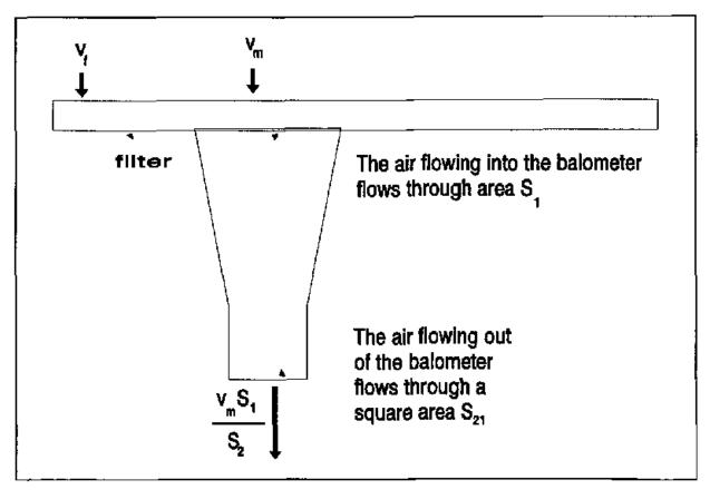
Figure C1. Schematic illustration of balometer used to measure the intake air flow in the ceiling of a booth
