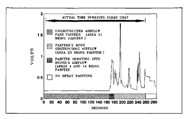
Figure 10 Analog output of Photovac Tip II when areas of the car are painted (for example Area 11 is the right side of the roof as shown in Figure 9)
