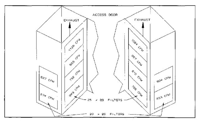
Figure 8 Airflow volume and distribution at the exhaust of the drive-thru booth
