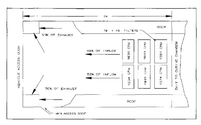
Figure 7 Airflow volume and distribution in the drive-thru booth
