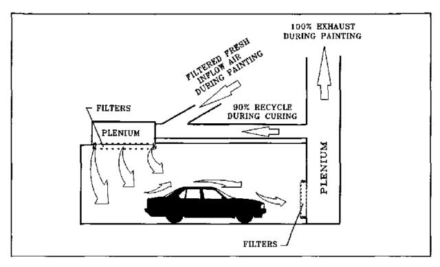
Figure 2 Semi-down draft booth and the general airflow pattern over and around a vehicle
