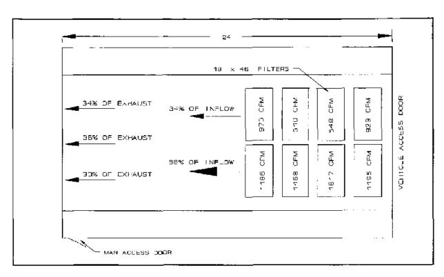
Figure 5 Airflow volume and distribution in the drive-in booth
