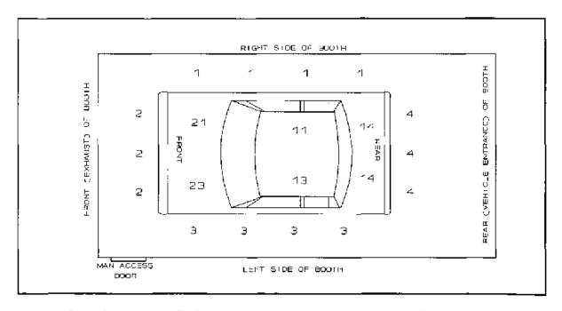
Figure 9 The areas of the car being painted (for example, Area II is the right side of the roof)
