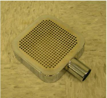
Figure 9: Rectangular side exhaust hood
