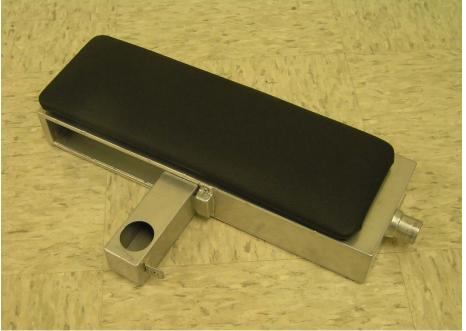
Figure 10: Hand rest exhaust
