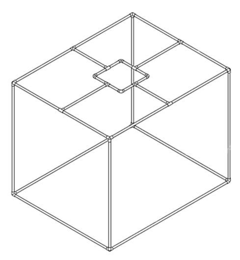
Figure 1: PVC frame layout for testing enclosure
