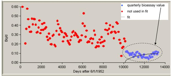
Figure B-6. 50th-percentile uranium urinalysis data used to estimate intakes of type S uranium occurring April 4, 1980 to December 31, 1988.
