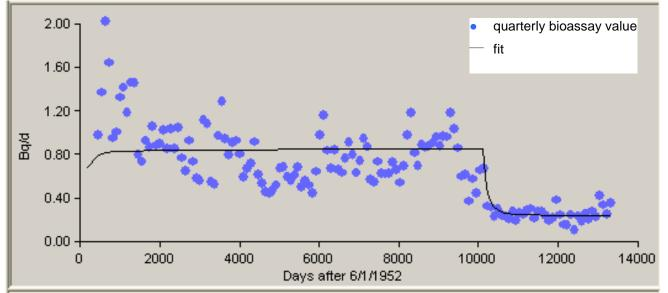
Figure B-4. 84th-percentile uranium urinalysis data used to estimate intakes of type M uranium occurring June 1, 1952, to December 31, 1988.
