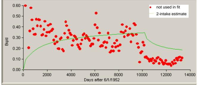
Figure B-7. Predicted 50th-percentile urinary excretion of type S uranium from 1952 to 1988 based on two independent intakes, compared with bioassay data.
