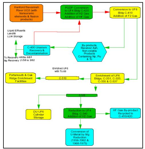
Figure 2-3. PGDP uranium enrichment process (Lockheed Martin 1997a).
