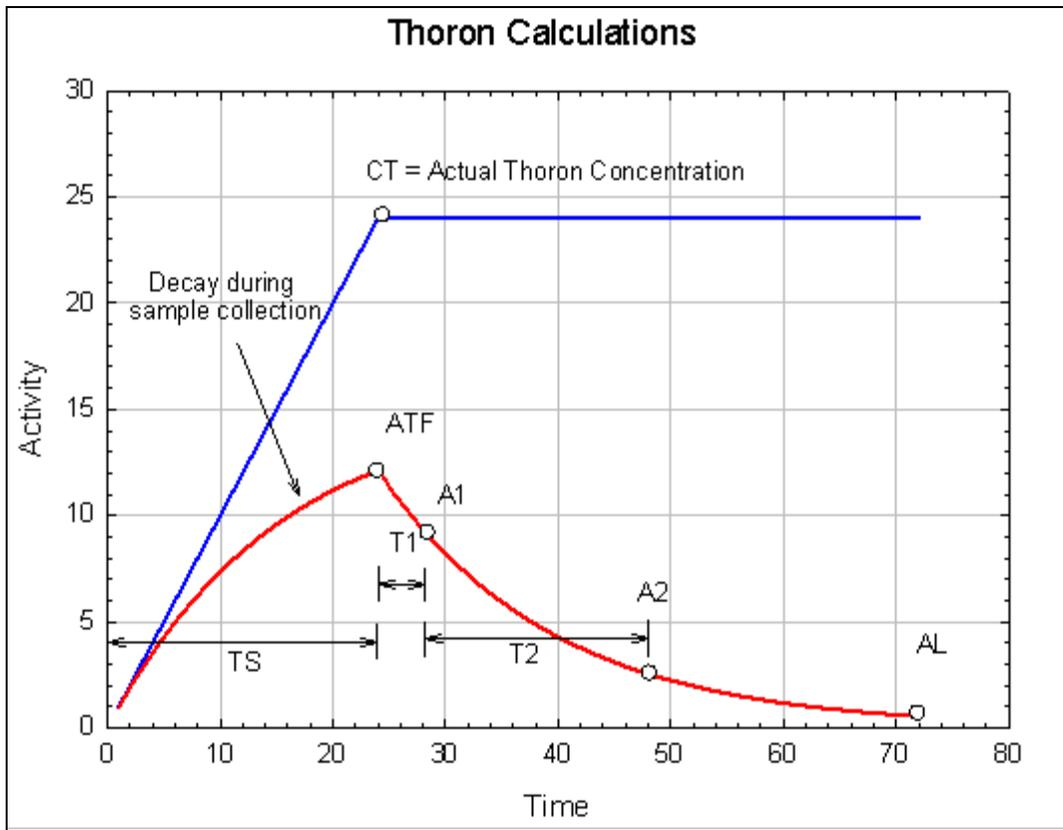
Figure 18. Kinetics of thoron decay illustrating time intervals used in Equations 1 through 8.
