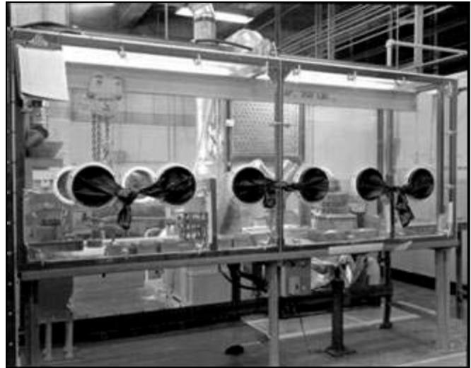
Figure 6. Thorium glovebox during operations. Source: Coughenour (2009). The photograph is unclassified and does not contain UCNI.
