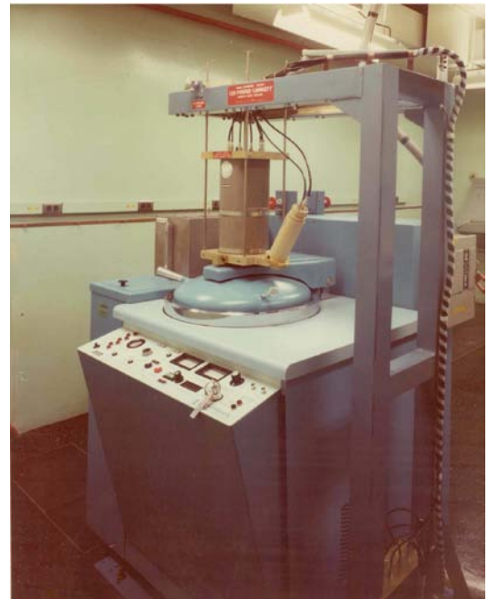
Figure 2-10. Spin tester (ORAUT-2006-0163).
