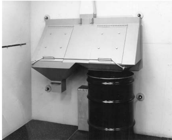
Figure 2-5. Boom box and collection container (ORAUT-2006-0163).
