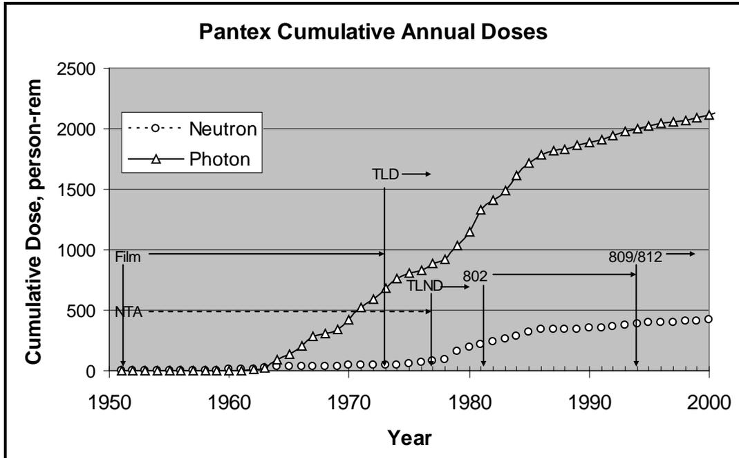
Figure 2-6. Evolution of external dosimetry at Pantex and a cumulative plot of annual photon and neutron recorded dose.
