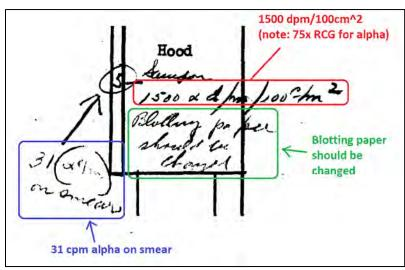
Figure 9 shows an alpha/beta/gamma contamination survey of the X-Cell which occurred in October 1961. As the figure shows, alpha contamination was found in several locations within the cell (sink, desk, bench, hood, table, and floor). Only one location within the X-Cell was noted to have beta/gamma
