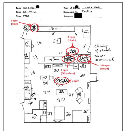
Figure 6. Example Alpha Survey of Rooms 212 and 216 in 1961 (CPP HP 1961)
