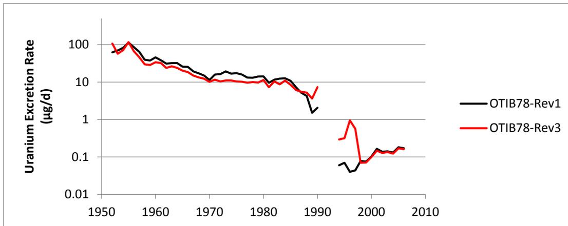
**Figure 4. Comparison of 84th Percentiles 1952 to 2006 (log scale)**
