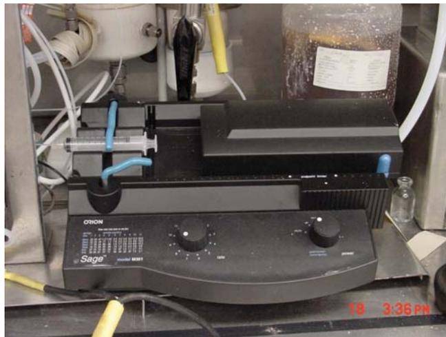
**Picture 4: Syringe pump, Sage Model M365**
