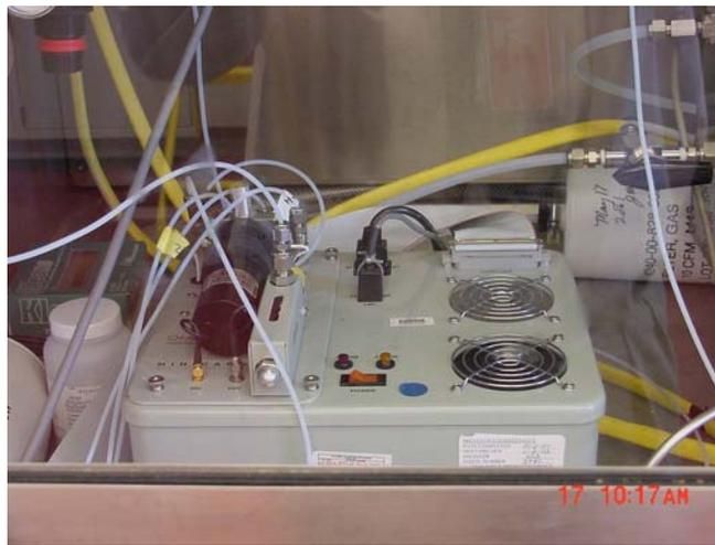
**Picture 3: MINIature Continuous Air Monitoring System, (MINICAMS)**
