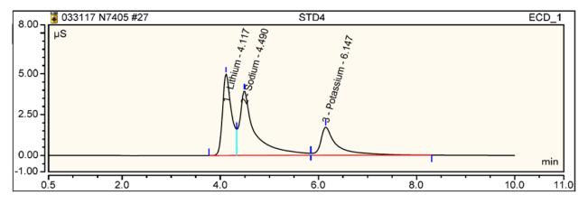
FIGURE 1. Chromatogram of standard solution containing Li, Na, and K.
