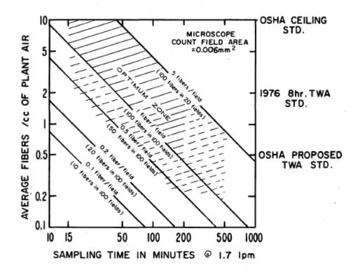
Figure 2 Optimum sampling times for airborne asbestos where microscopic field area =  $0.006 \text{ mm}^2$
