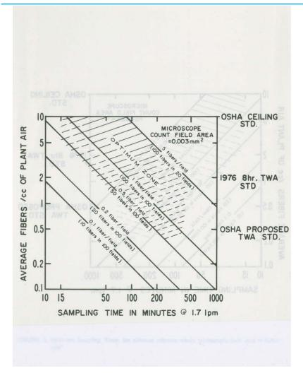
Figure 1 Optimum Sampling Times for airborne asbestos where microscopic field area = 0.003 mm<sup>2</sup>
