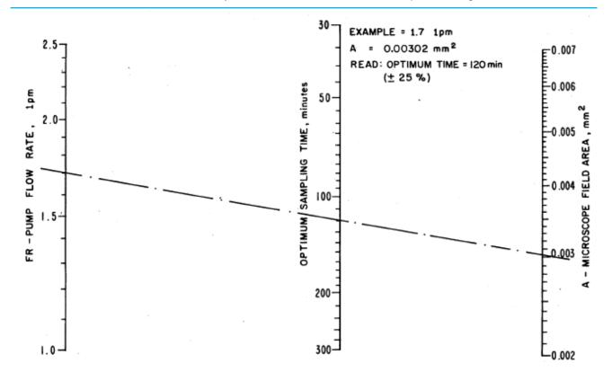
Figure 4 Nomogram of optimum sampling times for airborne asbestos fibers in concentrations of 1 to 10 fibers/cm<sup>3</sup>
