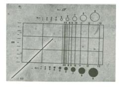
Figure 8 COUNT. One-half fiber. Fiber crosses bottom side and one end lies within count area.
