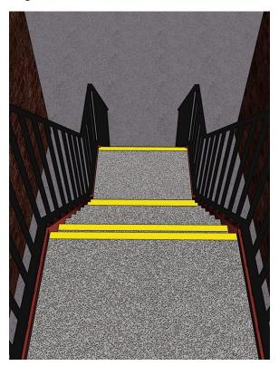
Figure 13. Painting of stair nosings before and after landings.
