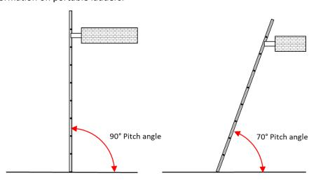
(L Q 3.2) You indicated that a single rail ladder is used. Install a double rail ladder rather than a single rail ladder as it is safer to use.
