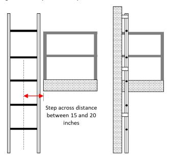
(L Q 7.6 or Q 7.7) You indicated that the top landing of the ladder is not adequately protected by a guardrail, chain, gate, or picket fence. It is preferable to treat the top landing of a ladder as a wall opening at that level. Install a self-closing gate, guardrail, chain, or picket fence at the top landing of the ladder. Routinely examine and maintain the guardrail, chain, gate, or picket fence to ensure that they are closed when not in use and are free from damage.
