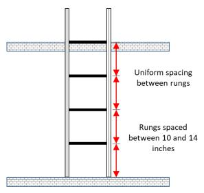
□ (L Q 5.5) You indicated that the lowest rung of the ladder is more than 14 inches from the floor. Install ladders with the first rung less than 14 inches from the walking surface to reduce the physical effort needed to gain access to the ladder. Routinely examine and maintain ladders.
