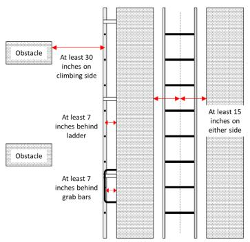
(L Q 4.5) You indicated that projections or obstructions are present on the climbing side (front) of enclosed ladders. Install ladders without any obstructions on the climbing side. No obstructions should be present within 15 inches from the centerline of the ladder on each side. Promptly remove/reroute any obstructions (such as cables, hoses, pipes, tools, or equipment) that result in clearances that are less than recommended. Routinely examine and maintain ladders and the surrounding area.
