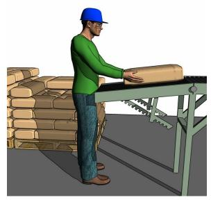
Figure 47. Worker standing at conveyor belt with an adjustable tilt end.
