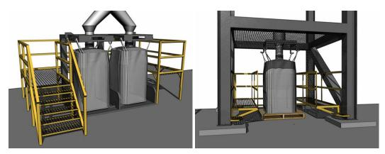
Figure 55. Platforms used to improve access to hooks and filling spout.
