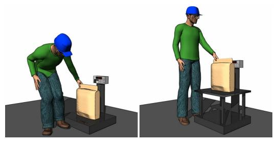
Figure 42. Scale placement on the ground requires worker to bend to pick up the bag from the scale (left). A table has been added on the scale to improve height and reduce bending required by workers (right).
