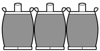
Figure 62. Example sizing of pallets for bulk bags: Pallets are approximately the same size as the bottom of the bag, and when placed side by side the filled bags touch (and the pallets do not touch).
