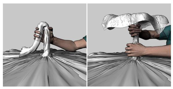
Figure 27. Snaking the liner of a bag (left) and flowering the liner of a bag (right).
