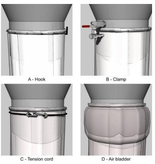
Figure 26. Methods of securing bag to filling spout.
