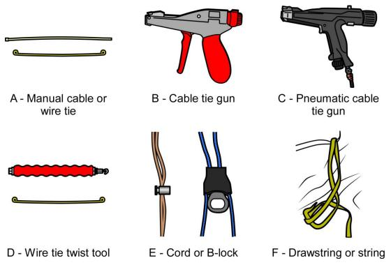
Figure 64. Methods of sealing bulk bags.
