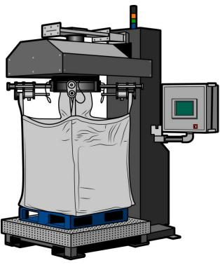
Figure 57. Example of filling station with rotating hooks.
