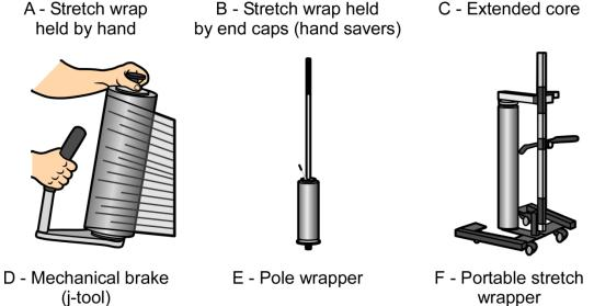
Figure 65. Tools used for stretch wrapping.
