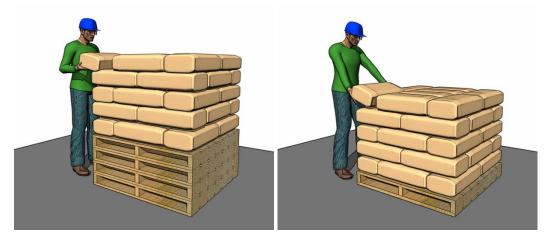
Figure 45. Method for using stacked pallets. Active pallet (fourth up from the ground on left) is placed on stack of inactive pallets and loaded until the top layer of bags is at 50 in from the ground (left), and pallet is moved by forklift to ground (right) and loading continues. Pallet on right should be loaded until the top layer of bags is 50 in from the ground.
