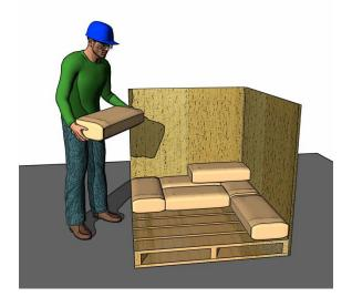
Figure 21. Corner frame used for palletizing.
