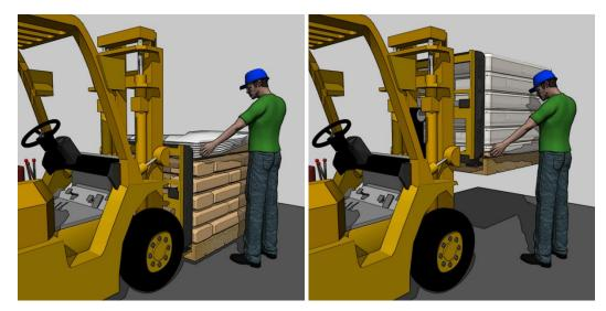
Figure 67. Forklift is used to raise pallet while worker stands still holding corners of shrink wrap. As the pallet is raised, the shrink wrap is pulled down over the stack of bags (beginning of process is shown on left; end is shown on right). As shown, this method does not require awkward reaching with the arms or bending/twisting the back.
