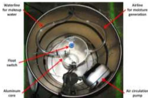
Fig. 2. Inside view of a simulated miner.
