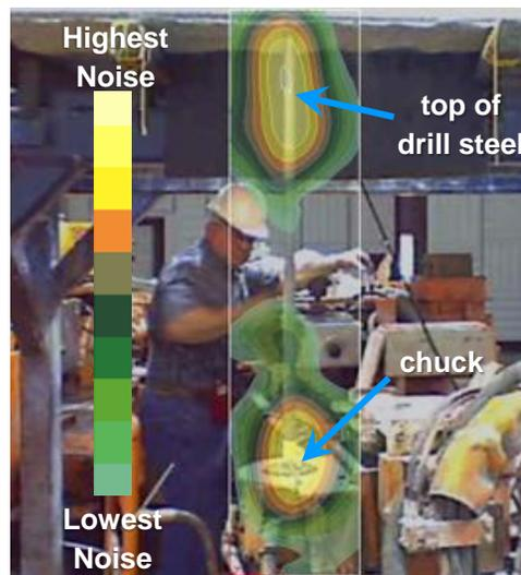
Figure 1. NIOSH's beamforming analysis showing dominant noise sources at the top of the drill steel and the drill chuck.
