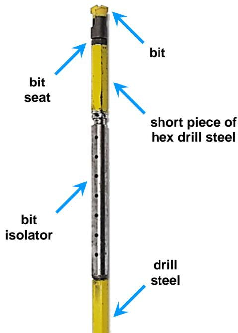
Figure 3. Drill bit isolator installed in a drill steel.
