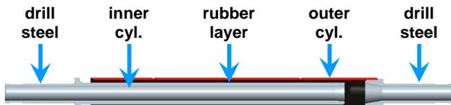
Figure 2. Drill bit isolator.
