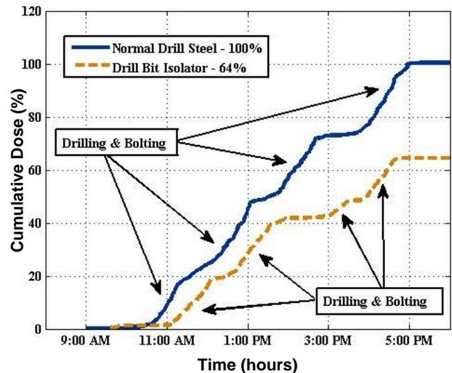
Figure 4. Operator noise exposure comparison shows reduction from 100% to 64%.
