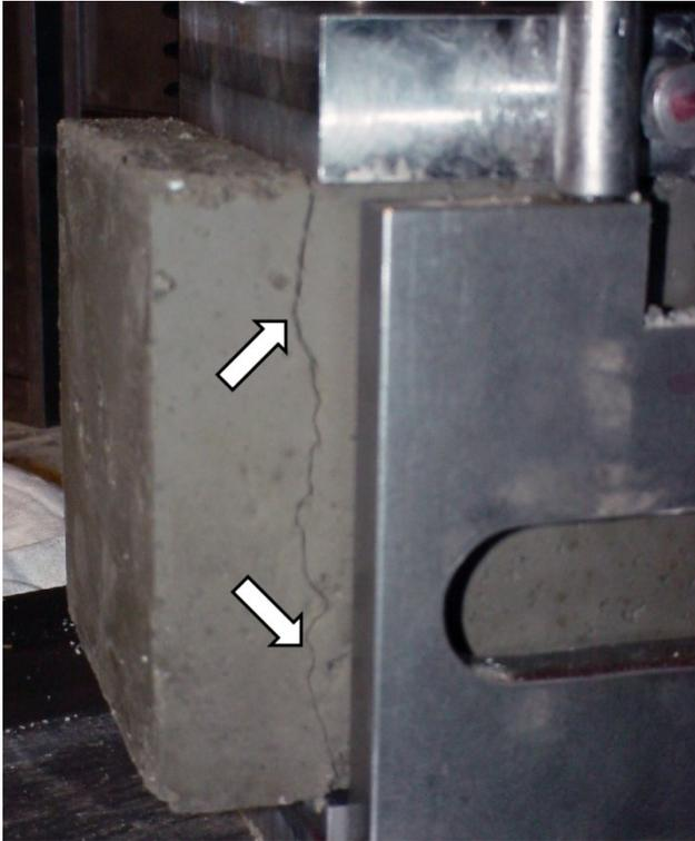
Figure 3. Vertical crack in shotcrete test specimen.
