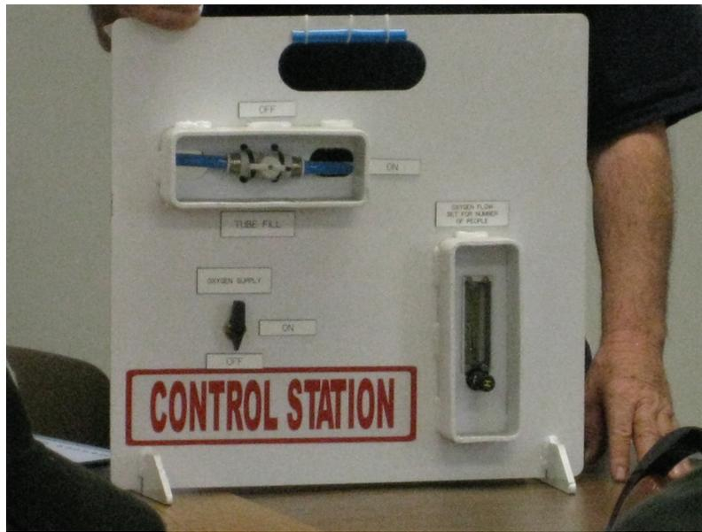
**Figure 4.** Mock-up of the internal oxygen controls and gauges on a refuge chamber.
