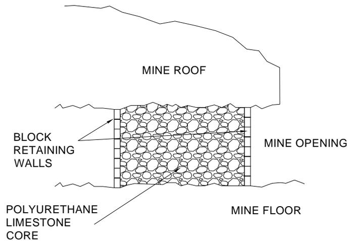
**Figure 3.—Grouted rock bulkhead installed across drift opening.**
